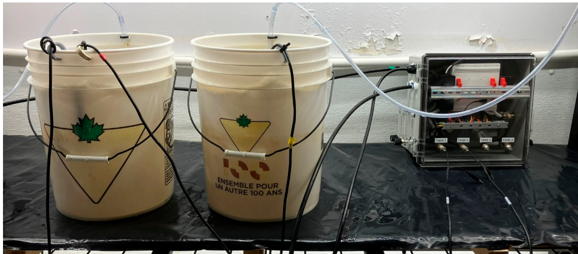
Figure 9. Experimental setup ((Left): Tank 1, (Middle): Tank 2, (Right): BREAD controller).
