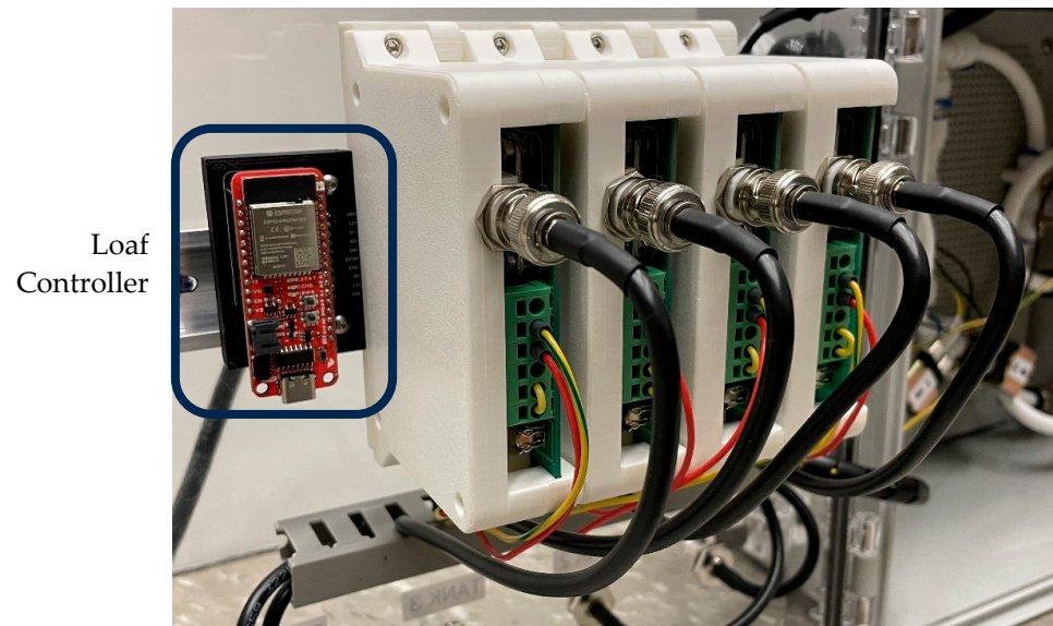
Figure 2. Loaf Controller connection configuration.
