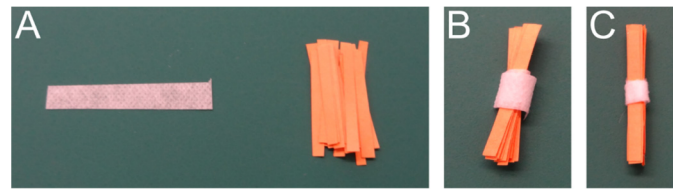
Figure 2. Bundling treatment. Results of CO 2 exposure on 20 bundles of bar-shaped paper samples (approximate paper width 1 mm): (A) bundle of paper and nonwoven fabric for bundling, (B) the bundled sample wreathed in nonwoven fabric; (C) the sample after treatment.
