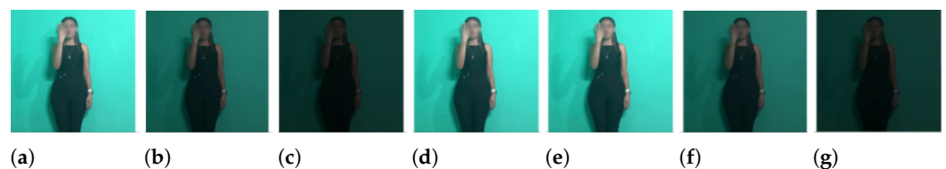
Figure 7. Illustrative example of the lighting and resolution conditions used for robustness analysis. From left to right: (a) original, (b) Light50 (approx. -1 EV), (c) Light25 (approx. -2 EV), (d) Res50 (spatial scale at 50%), (e) Res25 (25%), (f) Light50_Res50 (moderate combined), and (g) Light25_Res25 (severe combined).
