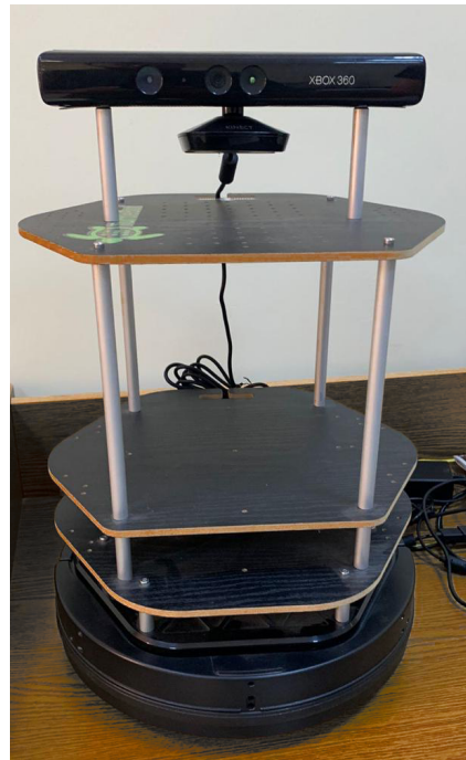
Figure 3. The Turtlebot2 robot platform.
