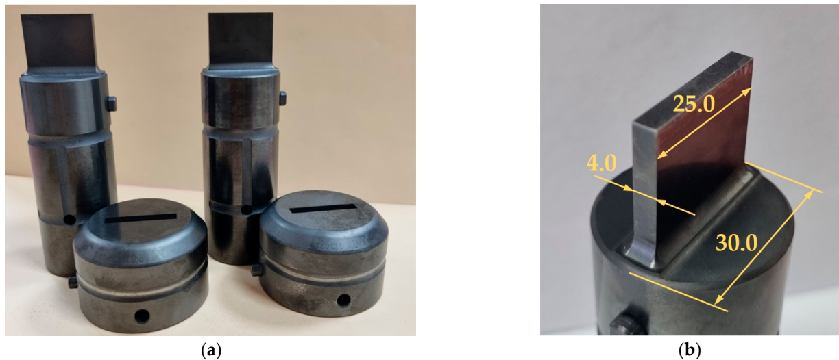
Figure 2. The design of the stamping tool (punch and die) (a) and the parameters of the working part of the punch (b).
