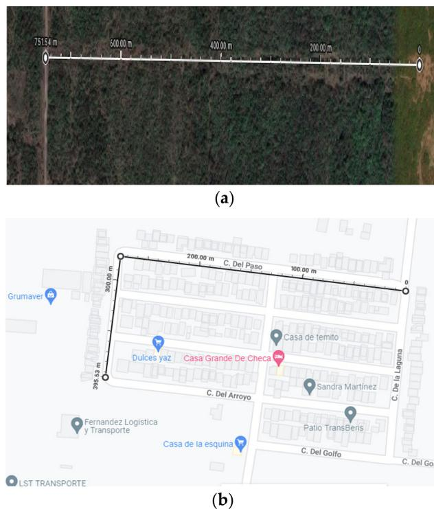
Figure 11. Maximum range obtained in (a) the open-field satellite image and (b) the city (19.233750,  $-96.210612$ ) for the proposed WSN.
