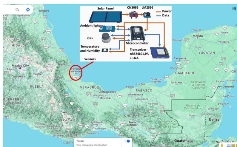
**Figure 1.** Localization of Veracruz and schematic view for each slave node of the proposed WSN.
