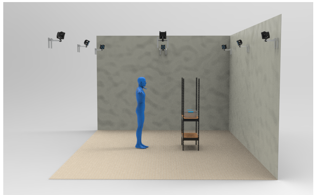
Figure 4. The motion analysis laboratory setup featuring an optoelectronic system alongside evaluation elements. The calibration volume dimensions were 5 m in length, 3 m in width, and 2 m in height.
