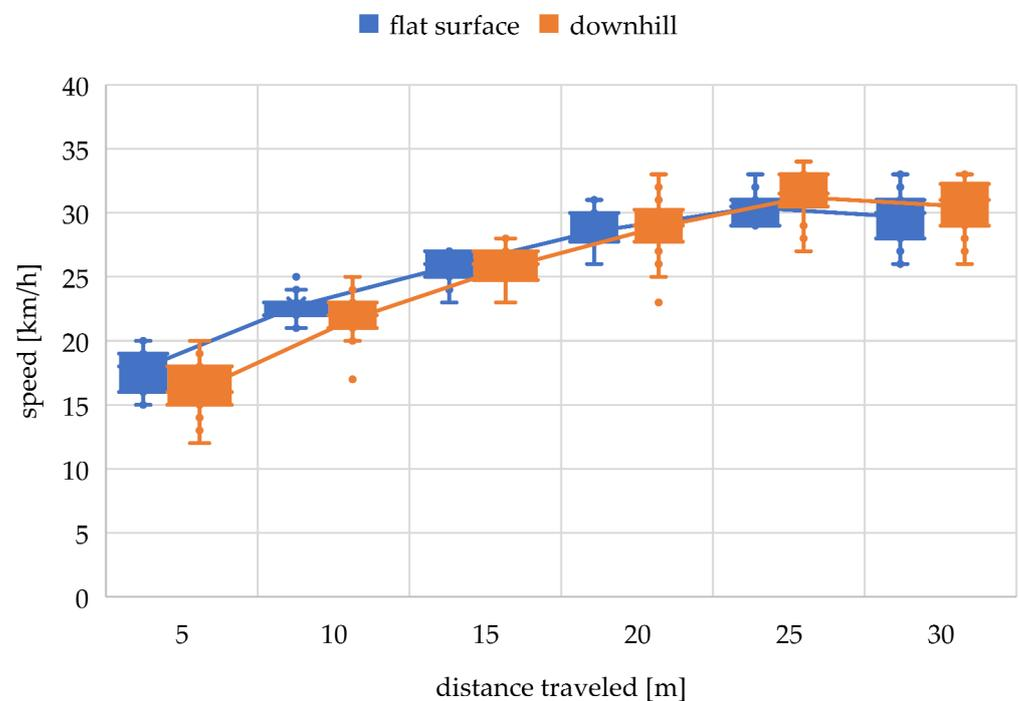
**Figure 2.** Comparison of speeds when driving on a flat surface and when driving downhill. Source: author.
