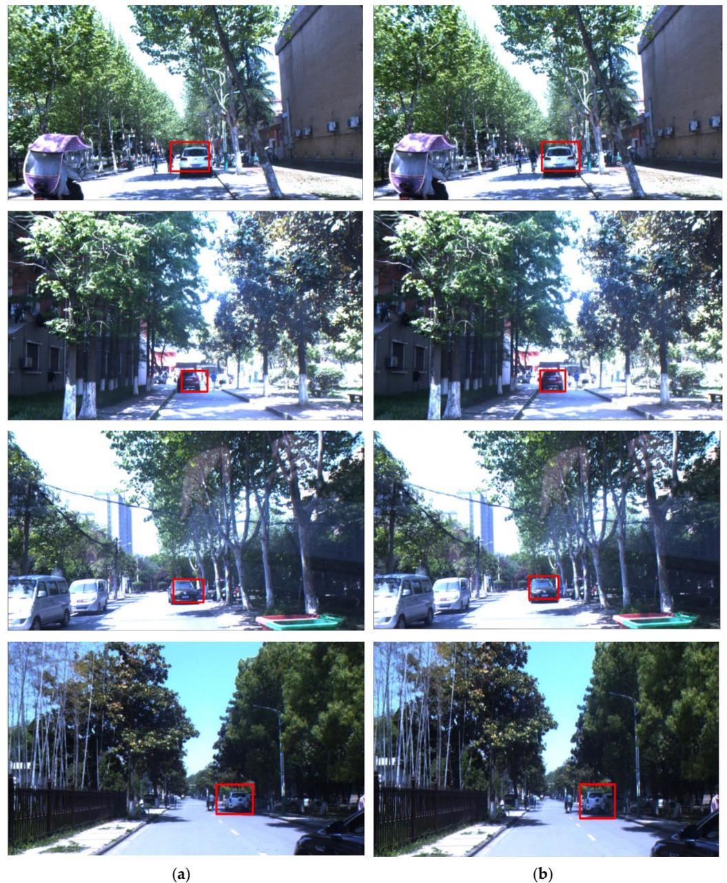
**Figure 15.** Comparison of vehicle recognition regions. (a) Initial radar identification region. (b) Identification region after improvement.
