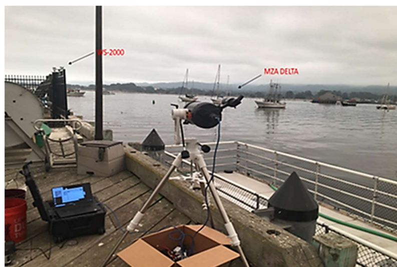
Figure 2. The laser propagation path over Monterey Bay, CA. The MZA DELTA transmitter is located on the Coast Guard Pier (upper left) and the target board is on a coastal bluff.
