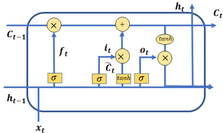
**Figure 2.** Architecture of Long short-term memory model. The notations of the graph are shown as follows.  $f_t, i_t, o_t$  are the forget gate, input gate and output gate.  $C_t$  is the cell state,  $\tilde{C}_t$  is the new candidate values,  $x_t$  is the input at time  $t$  and  $h_t$  is the hidden state.  $\times$  is the pointwise multiplication operation,  $+$  is the addition operation,  $\sigma$  is the sigmoid function and  $\tanh$  is the hyperbolic tangent function.
