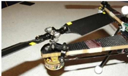
**Figure 17.** UAVs with variable pitch propellers [57].
