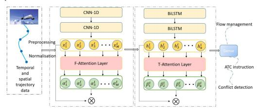
Figure 7. Architecture of the DA-CNN-BiLSTM hybrid model.
