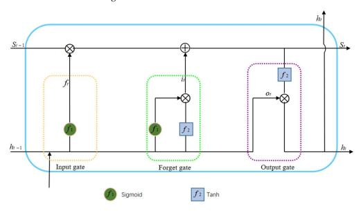
Figure 3. Structure of the LSTM.
