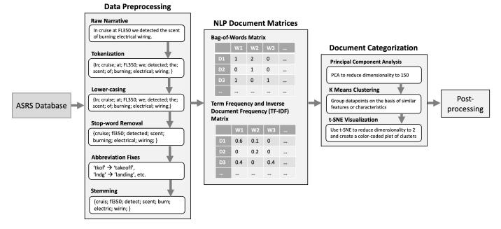
**Figure 1.** Methodology overview for data preprocessing, NLP implementation, and ASRS report classification leading up to post-processing (adapted from Ref. [37]).
