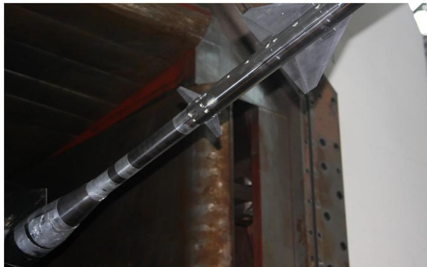
Figure 7. Support sting in wind tunnel test.
