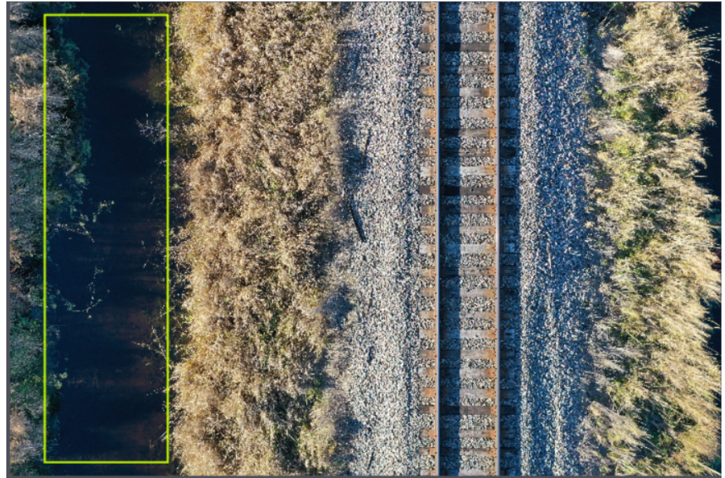
Figure 9. Example of water pooling.
