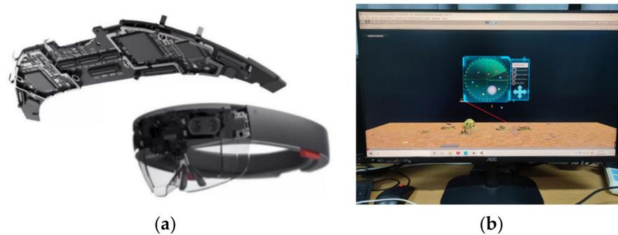
**Figure 1.** Display device ((a) Mixed reality display: HoloLens2; (b) Two dimensional display: AOC displayer).
