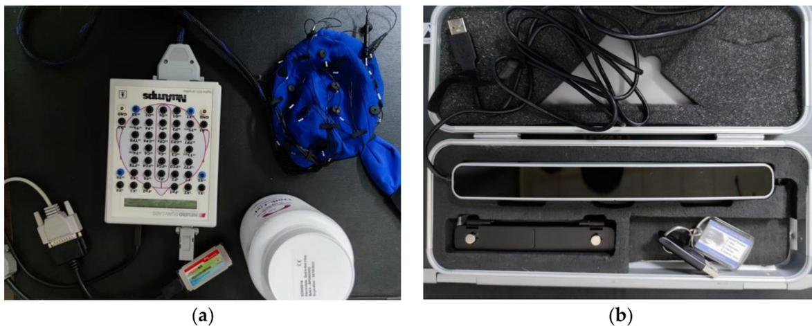
**Figure 2.** Experimental Test Setup ((a) Electroencephalograph; (b) Eye tracker).
