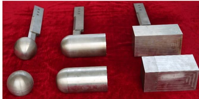
**Figure 7.** Models used in experiment on flows around debris in near space.
