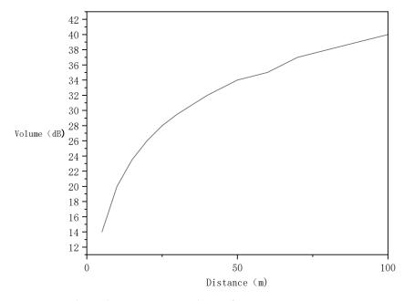
Figure 10. Volume distance correspondence of point source attenuation.
