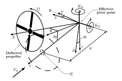
toward the direction of the freestream velocity,  $V_{\infty}$ , and horizontally supported by a pylon pivoted on the wing.
