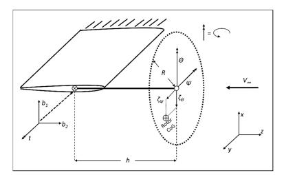
Figure 4. Gimballed hub model schematic.
