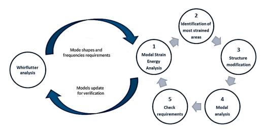
Figure 5. Aeroelastic tailoring process scheme.
