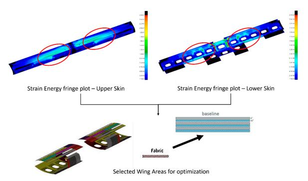
Figure 7. Identification of wing areas for torsional stiffness improvement.
