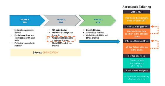
Figure 1. T-WING design and aeroelastic tailoring phases.
