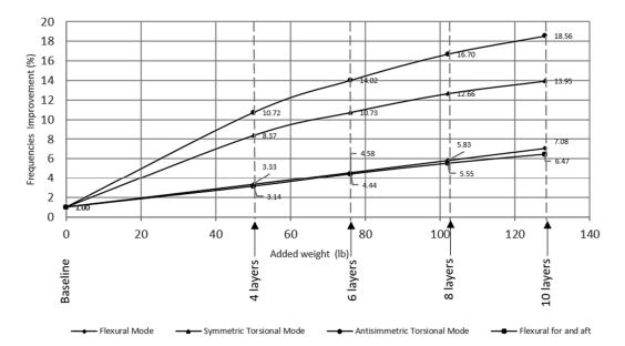
Figure 8. Airplane Mode Flexural and Torsional Frequencies vs. Added Mass.
