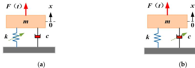
**Figure 3.** Typical schematic diagram of a semi-active vibration isolation system: (a) variable stiffness; (b) variable damping.
