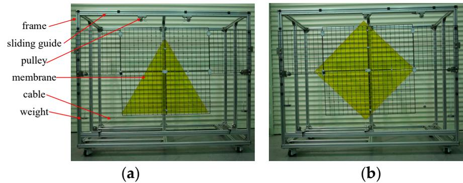
**Figure 9.** Test piece system: (a) square membrane; and (b) trapezoidal membrane.
