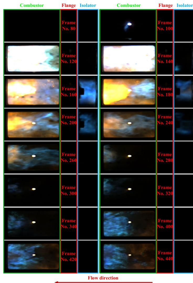
Figure 6. High-speed images of the ignition process of Case #1. (Original images).
