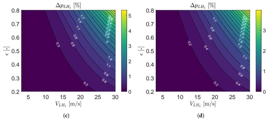
**Figure 15.** Intercooler HE, pressure drop of LH<sub>2</sub> at the HE outlet for varying effectiveness and flow velocity at the inlet of the HE tubes at the design point. (a) Take-off, (b) top of climb, (c) initial cruise, and (d) end of cruise operating conditions.
