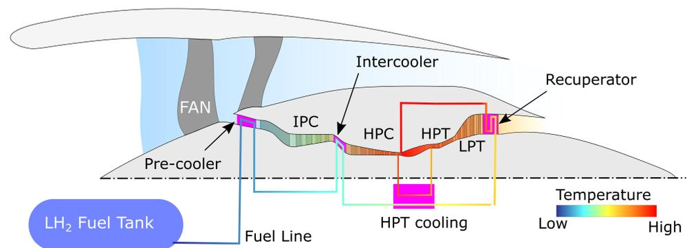
**Figure 1.** Cross-sectional meridional cut of a turbofan engine, including possible locations for core heat rejection to the hydrogen fuel. The fuel is stored at its boiling point in the cryogenic tank. The temperature of the hydrogen in the fuel line is increased by the different core-installed heat exchangers on its way to the combustion chamber. IPC: Intermediate-pressure compressor; HPC: High-pressure compressor; HPT: High-pressure turbine; LPT: Low-pressure turbine.
