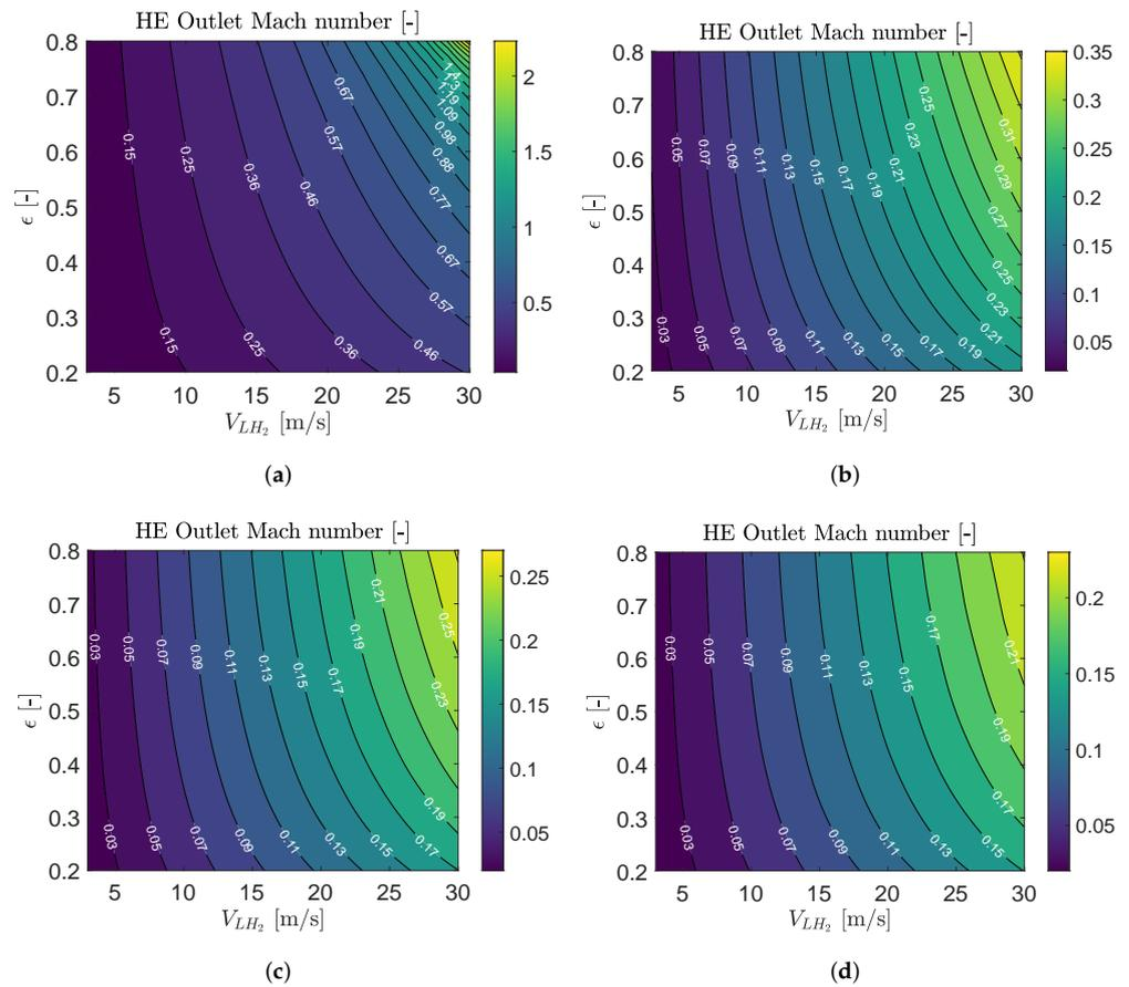
**Figure 10.** Precooler HE performance parameter at the end-of-cruise condition Mach number of LH<sub>2</sub> at the HE outlet for varying effectiveness and flow velocity at the inlet of the HE tubes at the design point. (a) Take-off, (b) top of climb, (c) initial cruise, and (d) end of cruise operating conditions.
