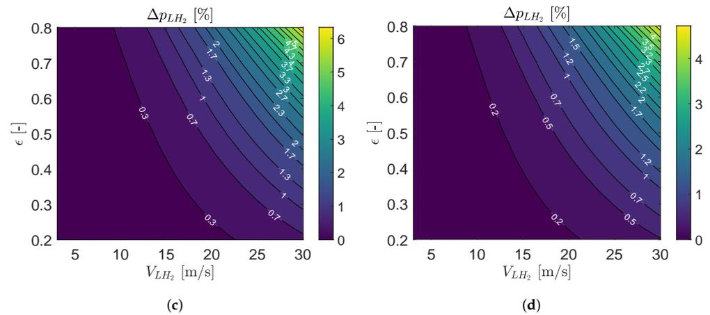
**Figure 11.** Precooler HE, pressure drop of LH<sub>2</sub> at the HE outlet for varying effectiveness and flow velocity at the inlet of the HE tubes at the design point. (a) Take-off, (b) top of climb, (c) initial cruise, and (d) end of cruise operating conditions.
