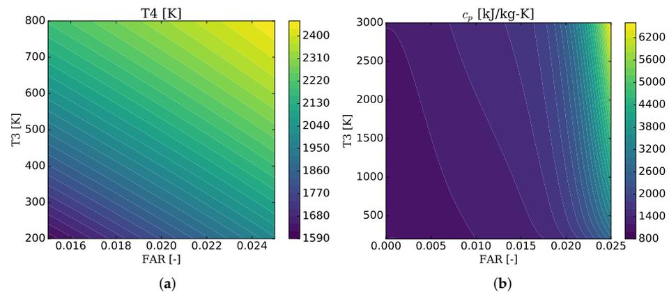
**Figure 2.** Temperature and FAR (fuel–air ratio) dependent tables for H<sub>2</sub> combustion products at 1 bar. (a) Combustion exit temperature; (b) specific heat at constant pressure.
