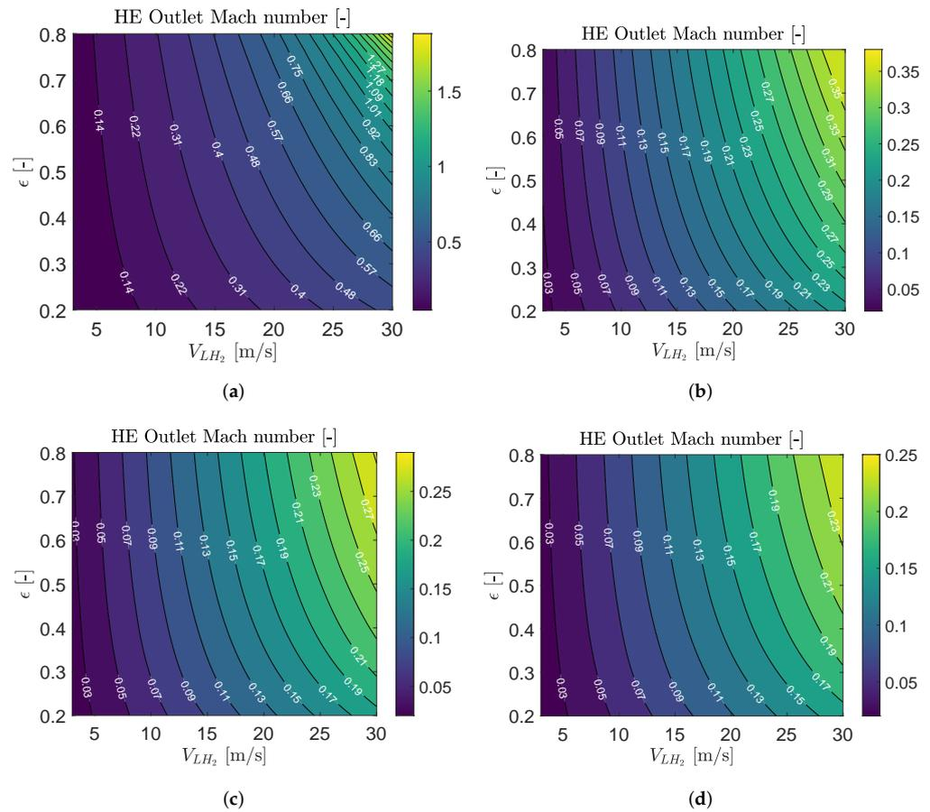
**Figure 14.** Intercooler HE, Mach number of LH<sub>2</sub> at the HE outlet for varying effectiveness and flow velocity at the inlet of the HE tubes at the design point. (a) Take-off, (b) top of climb, (c) initial cruise, and (d) end of cruise operating conditions.
