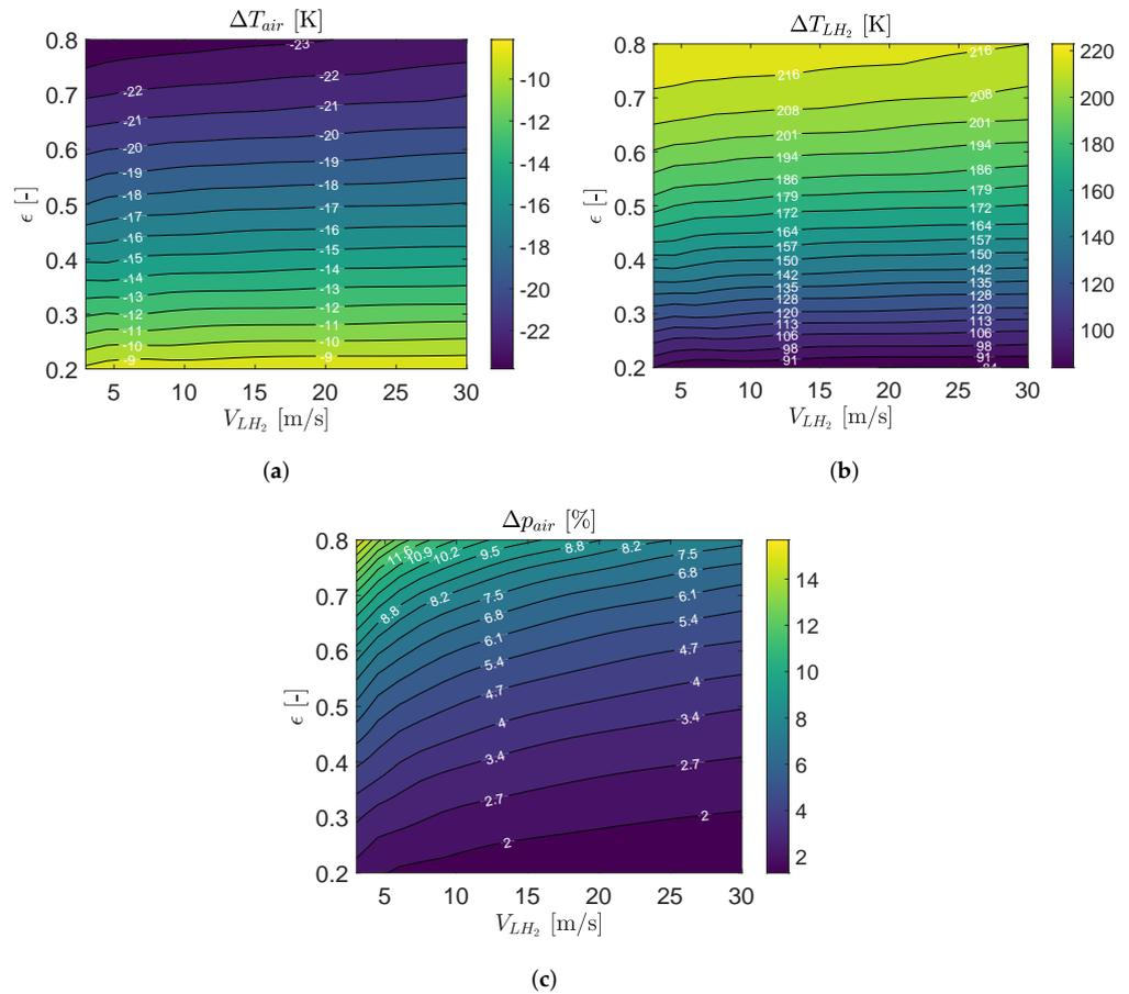
**Figure 8.** Pre-cooler HE performance parameters at the end-of-cruise condition: (a,b) temperature difference, and (c) pressure drop percentage across the HE tubes, for varying HE effectiveness and flow velocity at the inlet of the HE tubes at the design point.
