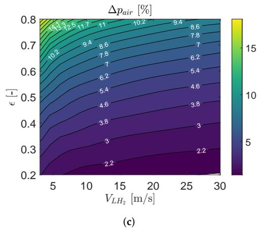
**Figure 12.** Intercooler HE performance parameters at the end-of-cruise condition: (a,b) temperature difference, and (c) pressure drop percentage across the HE tubes, for varying HE effectiveness and flow velocity at the inlet of the HE tubes at the design point.
