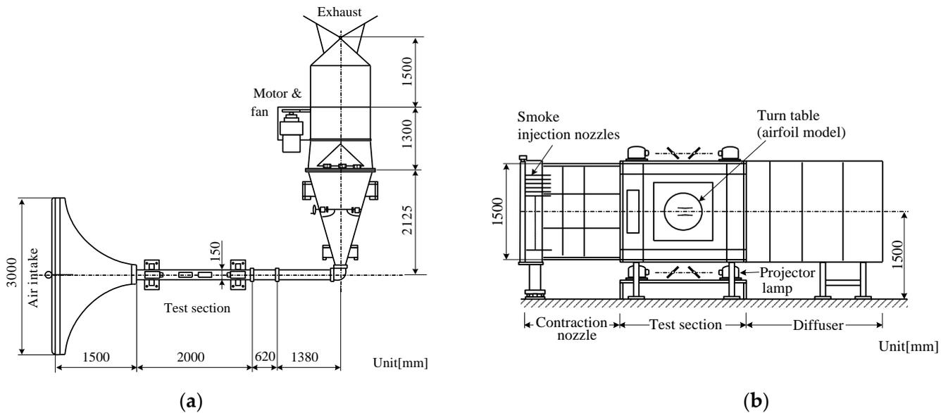
**Figure 1.** Overview of the low-speed wind tunnel: (a) top view; (b) side view.
