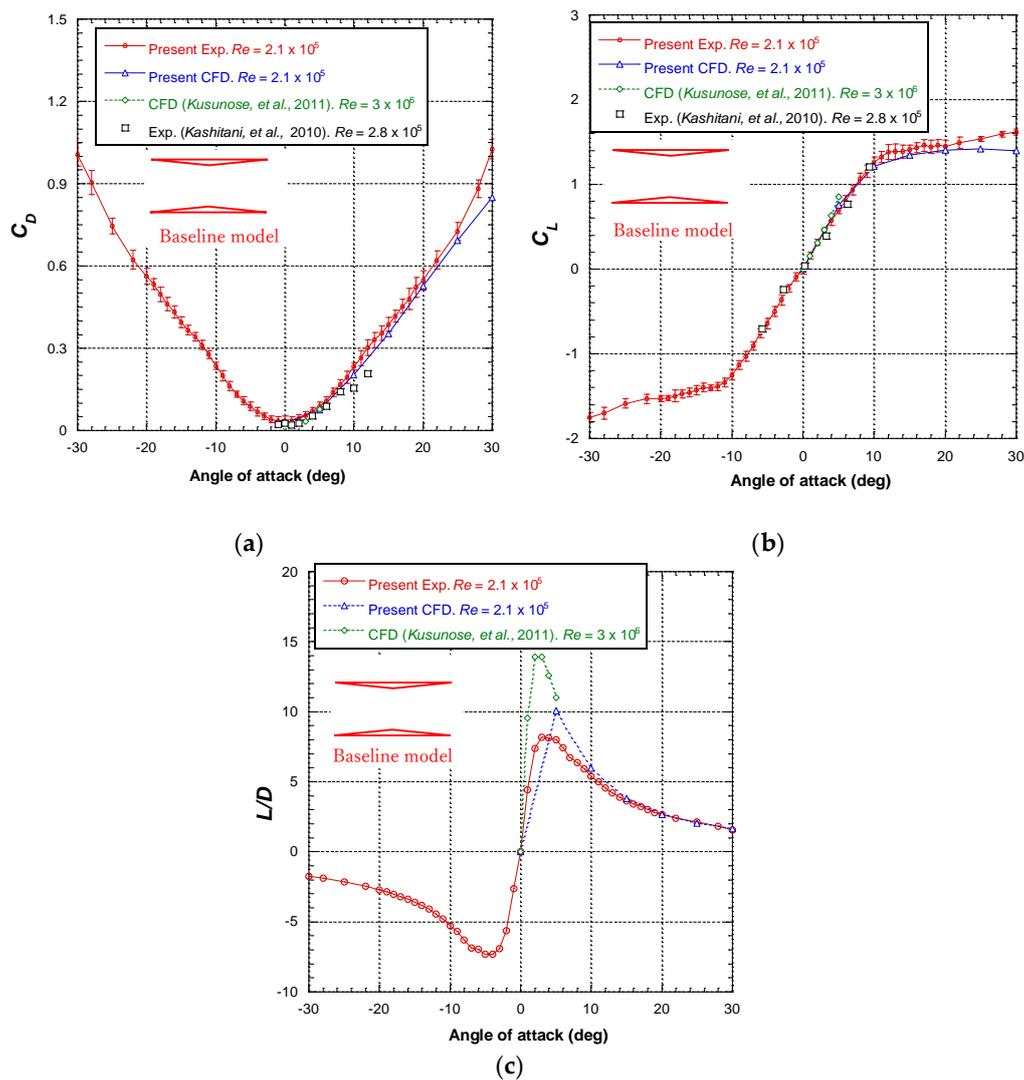
**Figure 6.** Aerodynamic characteristics of the baseline model: (a) drag coefficient; (b) lift coefficient; (c) lift-to-drag ratio.
