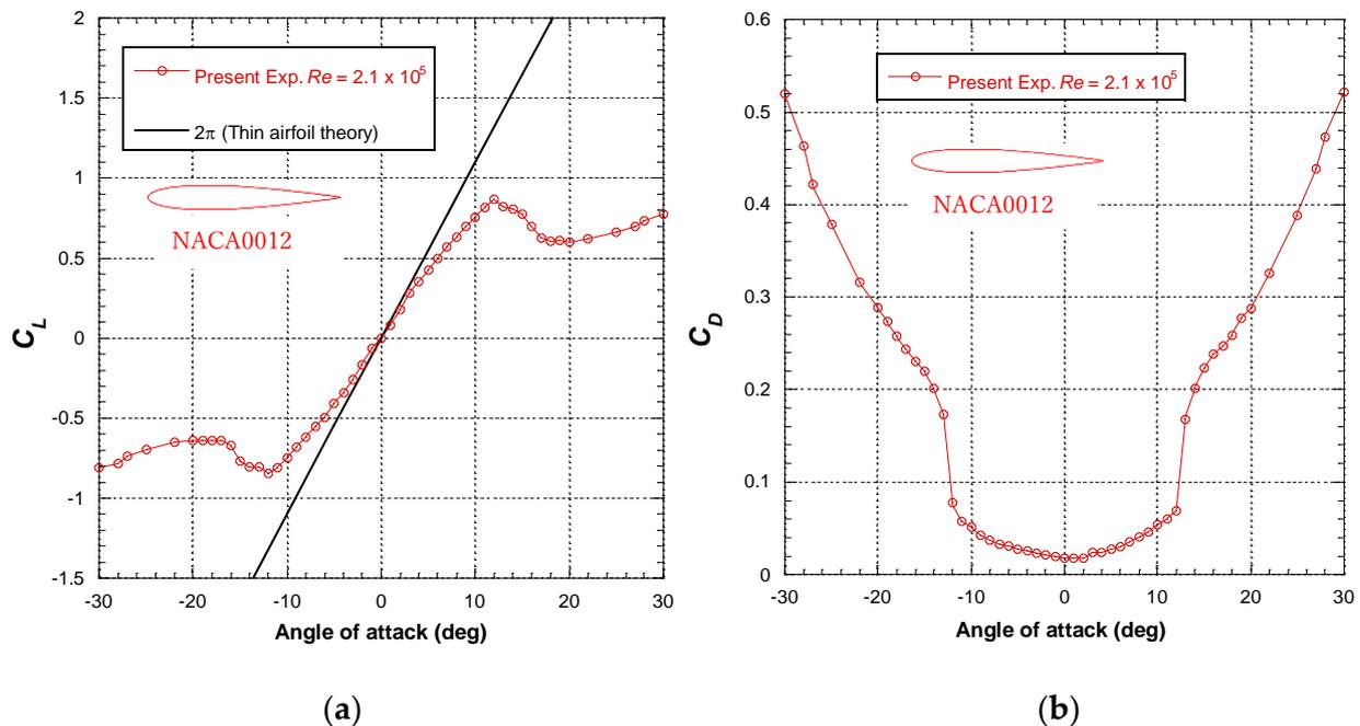
**Figure 5.** Results of single NACA0012 for balance measurement: (a) drag coefficient; (b) lift coefficient.
