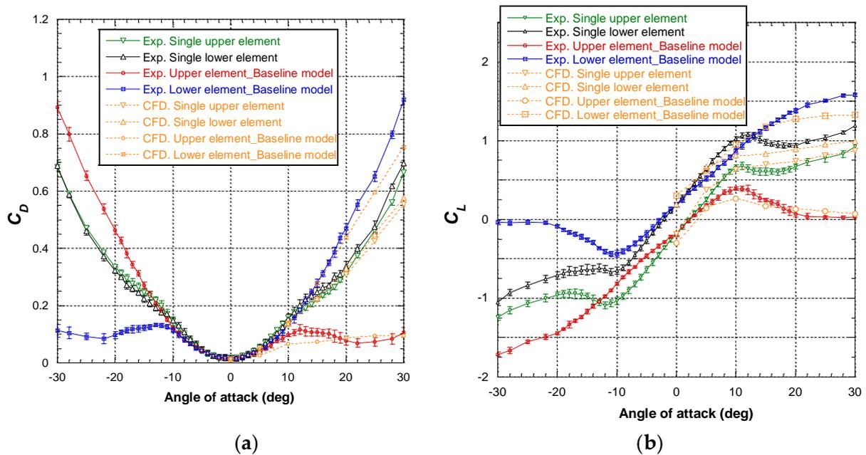
**Figure 7.** Comparison of aerodynamic characteristics of the wing elements as single configuration and baseline configuration: (a) drag coefficient; (b) lift coefficient.
