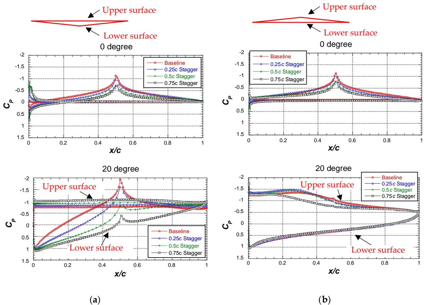
**Figure 11.** Comparison of pressure coefficient in airfoil surface of the staggered biplane configuration (CFD results): (a) upper element; (b) lower element.
