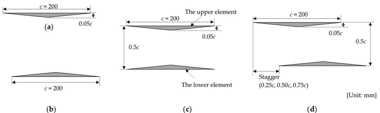
**Figure 3.** Experimental models: (a) single upper element; (b) single lower element; (c) baseline model (Busemann biplane—no stagger); (d) staggered models (three stagger lengths).
