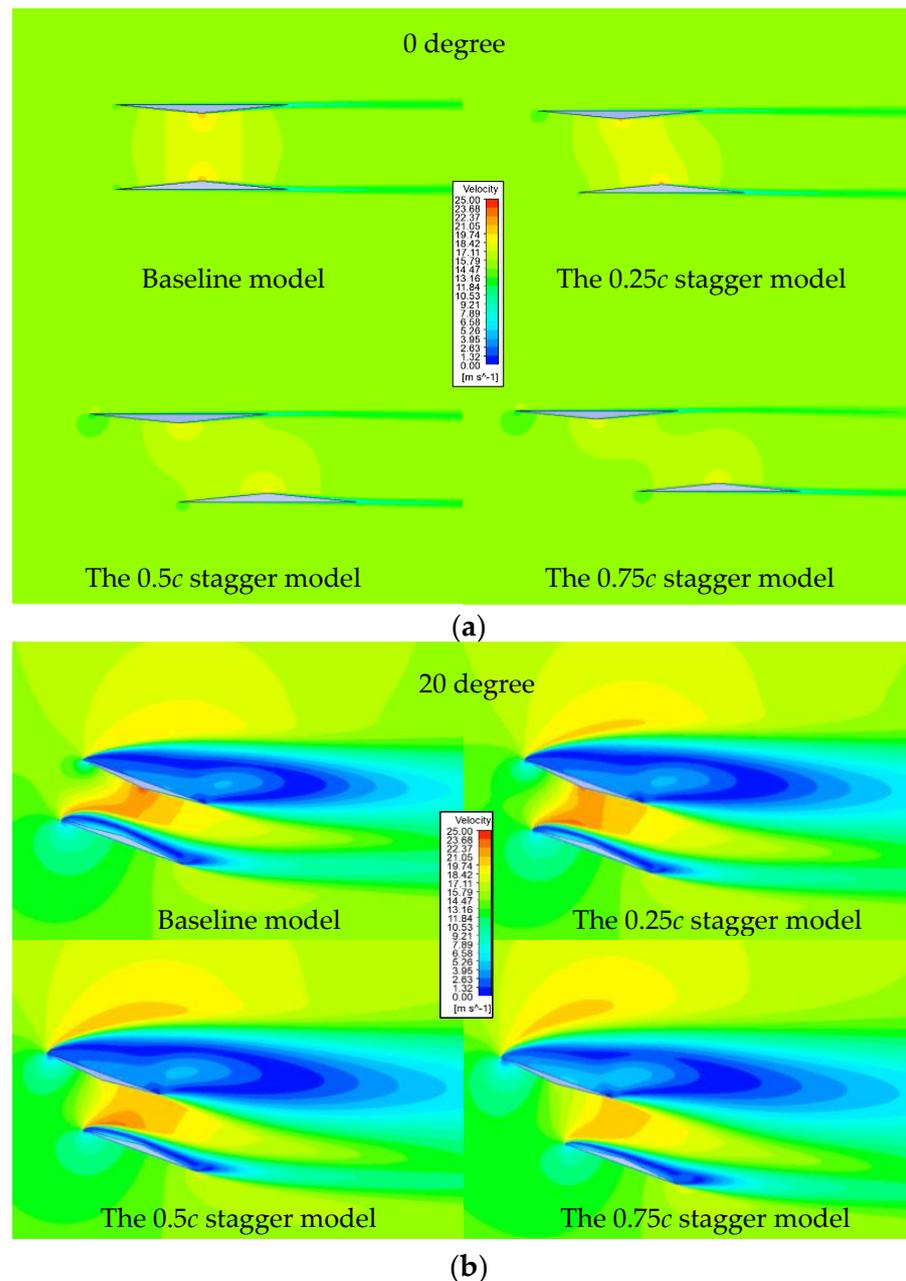
**Figure 12.** Velocity distributions around the staggered biplane configuration (CFD results): (a) 0 degrees; (b) 20 degrees.
