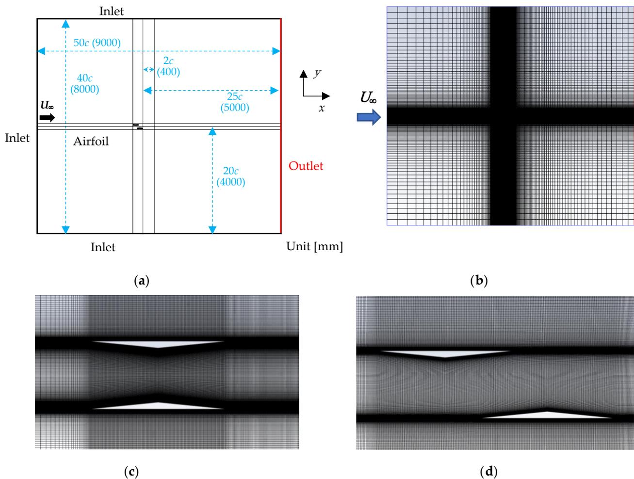
**Figure 4.** Meshes used for numerical calculations: (a) computational domain; (b) overview of grid; (c) grid distribution around the baseline model; (d) grid distribution around the 0.75c stagger model.
