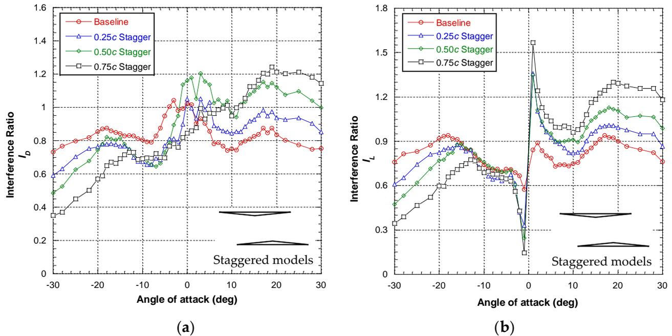
**Figure 10.** Interference ratios of the biplane aerodynamic forces: (a) drag interference ratio; (b) lift interference ratio.
