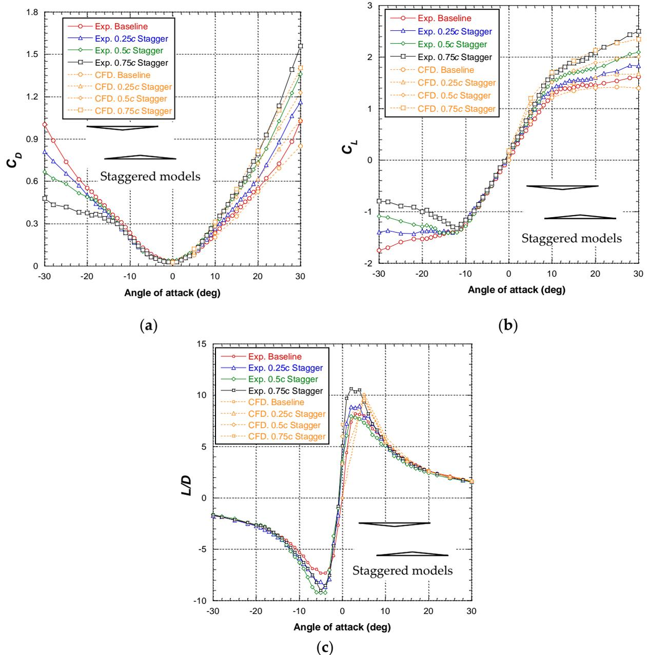
**Figure 8.** Effect of stagger on aerodynamic characteristics: (a) drag coefficient; (b) lift coefficient; (c) lift-to-drag ratio.
