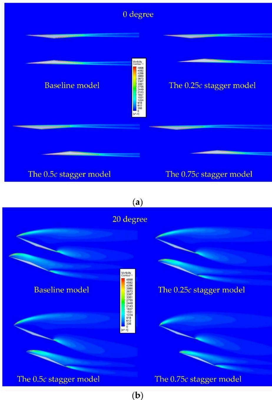
**Figure A5.** Vorticity distributions around the staggered biplane configuration (CFD results): (a) 0 degrees; (b) 20 degrees.
