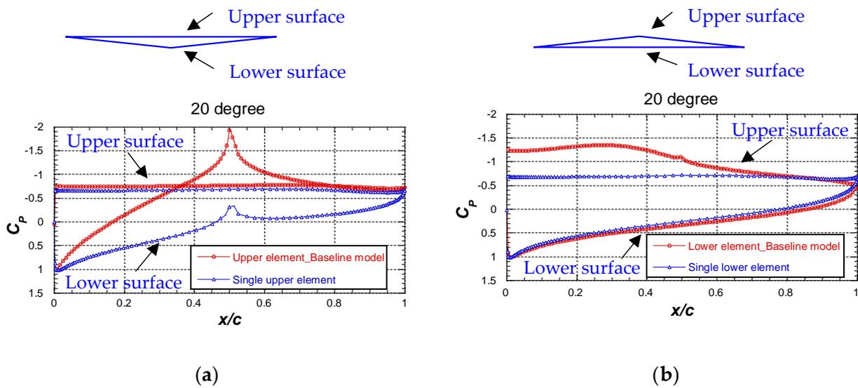
Figure A3. Comparison of pressure coefficient in airfoil surface of the wing elements as single configuration and baseline configuration (CFD results): (a) upper element; (b) lower element.
