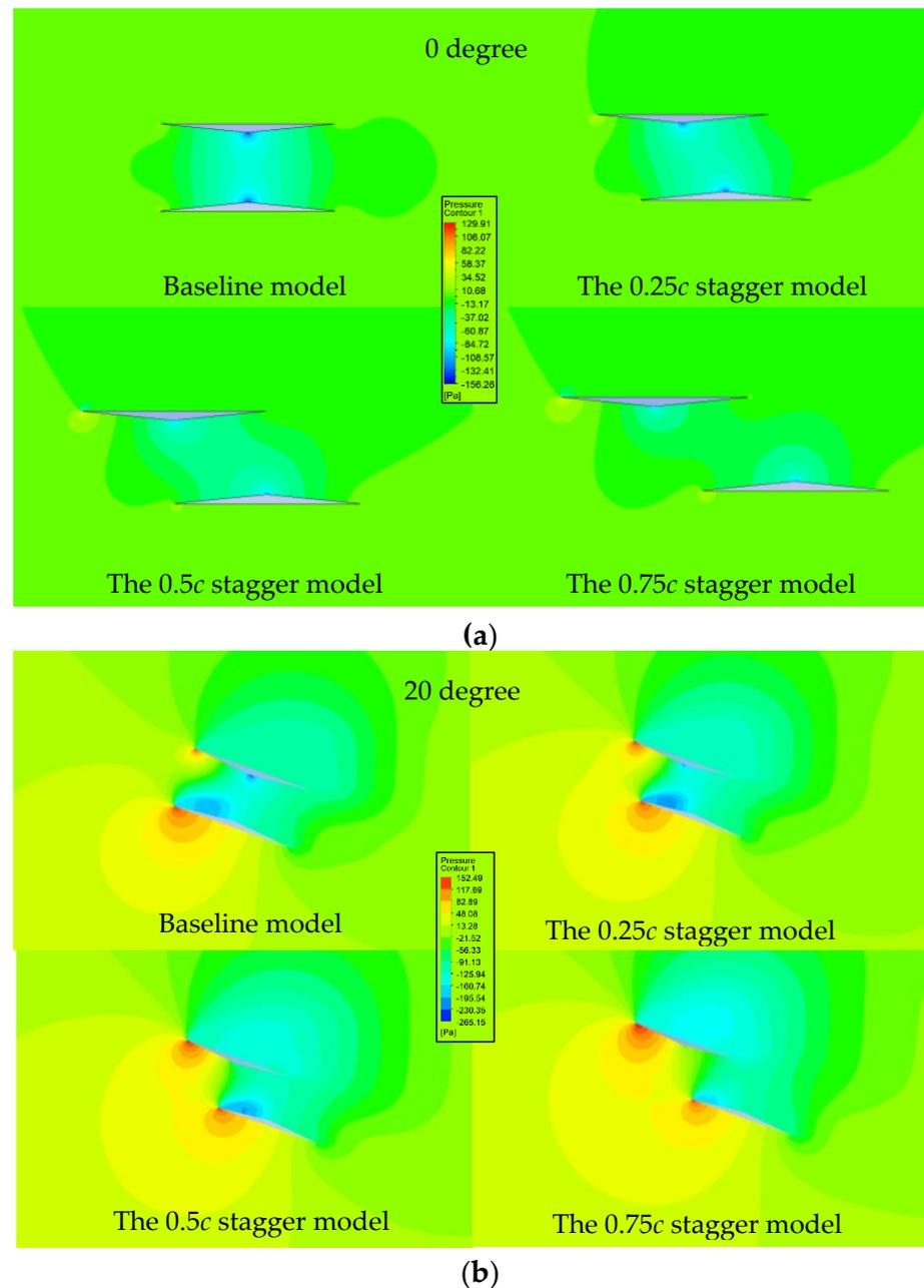
**Figure 13.** Pressure distributions around the staggered biplane configuration (CFD results): (a) 0 degrees; (b) 20 degrees.
