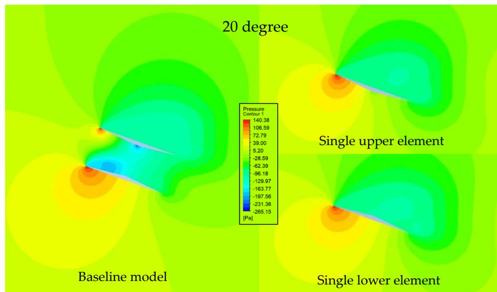
Figure A4. Pressure distributions around the wing elements as single configuration and the baseline configuration (CFD results) at 20 degrees.
