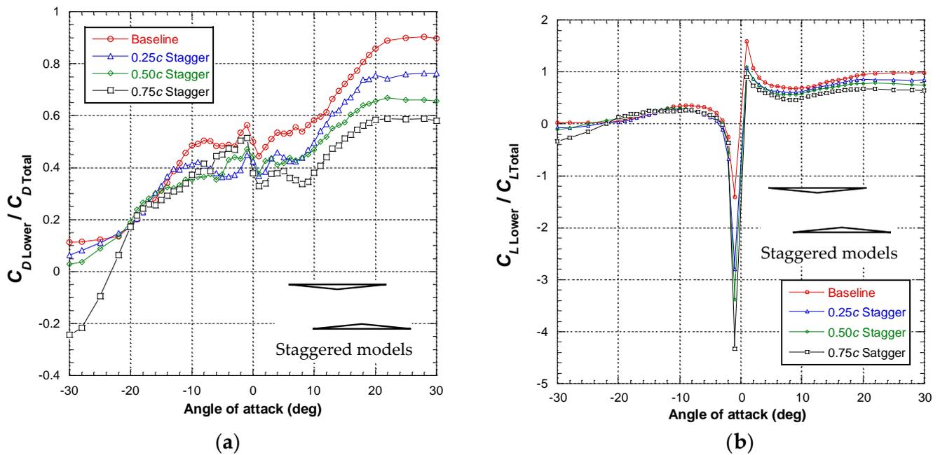
**Figure 9.** Ratios of the lower wing to the biplane performances: (a) ratio for drag coefficient; (b) ratio for lift coefficient.
