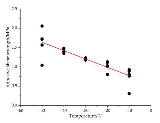
Figure 20. Adhesion shear strength of freshwater sample with salinity of 0‰.
