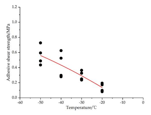
Figure 18. Adhesion shear strength of Dalian seawater sample with salinity of 5.0‰.
