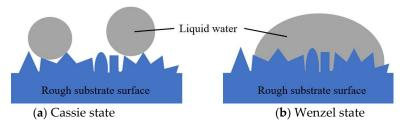
Figure 17. Contact between liquid water and rough substrate surface. Adapted from ref. [5].
