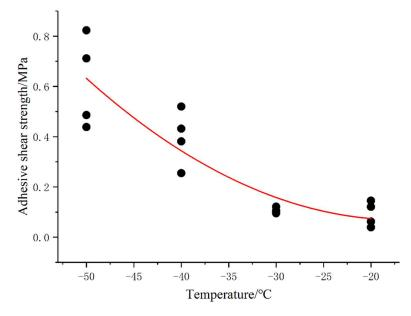
Figure 12. Adhesion shear strength of Dalian seawater sample.
