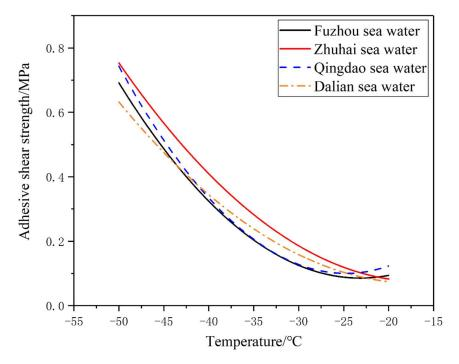
Figure 16. Comparison of adhesion shear strength of different seawater samples.
