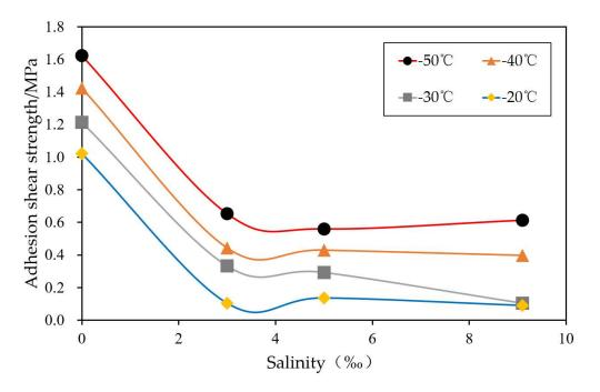
**Figure 22.** Relationship between adhesion shear strength and salinity of water samples at different temperatures.
