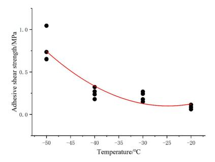
Figure 13. Adhesion shear strength of Qingdao seawater sample.
