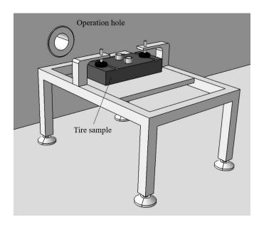
Figure 4. Tire-sample-clamping device.
