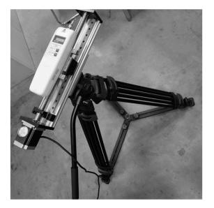
Figure 5. Tensile-force measurement system.
