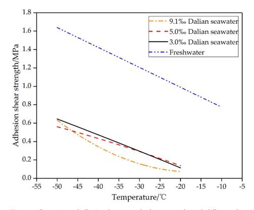
Figure 21. Comparison of adhesion shear strength of water samples with different salinities.
