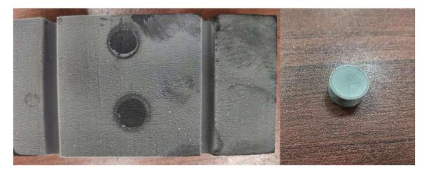
**Figure 11.** Tire sample and sea ice sample after the test (Zhuhai seawater sample, -30 °C).
