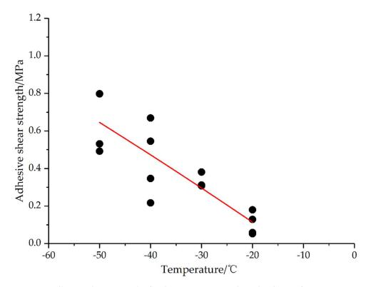
Figure 19. Adhesion shear strength of Dalian seawater sample with salinity of 3.0‰.
