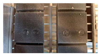
**Figure 23.** Tire-sample surface after freshwater static icing test (-50 °C).
