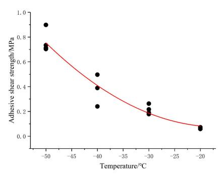
Figure 15. Adhesion shear strength of Zhuhai seawater sample.
