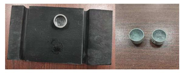
**Figure 10.** Tire sample and sea ice sample after the test (Zhuhai seawater sample, -20 °C).
