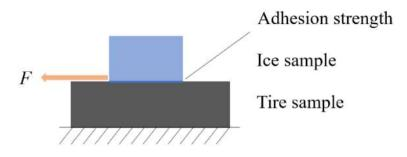
Figure 2. Mechanical model.
