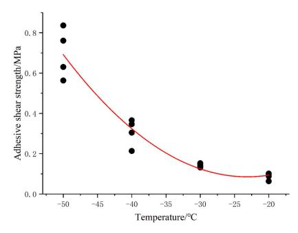
Figure 14. Adhesion shear strength of Fuzhou seawater sample.
