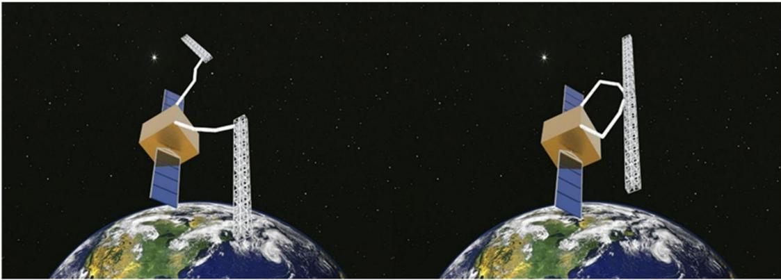
**Figure 1.** Assembling modular components using a dual-arm space robot with flexible appendages.
