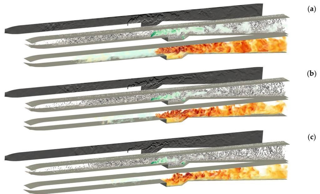
**Figure 6.** Perspective views of the flow in terms of the refraction index gradient,  $\nabla n$ , the 2nd invariant of the velocity gradient,  $\lambda_2$  (gray), and the  $H_2$  mass-fraction (green), and the temperature,  $T$  (warm colors), for (a) Case F1, (b) Case F3, and (c) Case F5.
