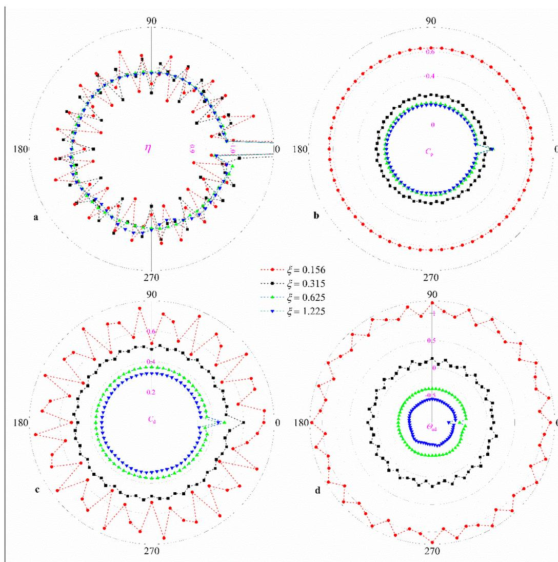
**Figure 12.** Distribution of (a) mass-flow-rate ratio  $\eta$ , (b) total-pressure-loss coefficient  $C_p$ , (c) discharge coefficient of holes  $C_d$ , and (d) adiabatic effectiveness  $\Theta_{ad}$  for different area ratios of nozzles to holes  $\xi$ .
