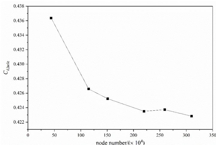
**Figure 6.** The grid-independent solution,  $\lambda_{T,P} = 0.236$ ,  $\beta_p = 0.96$ .
