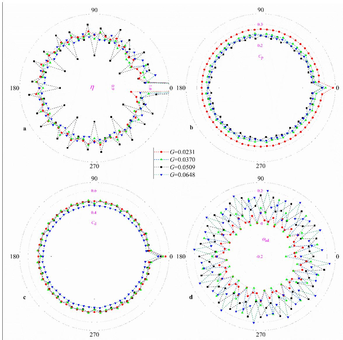
**Figure 15.** Distribution of (a) mass-flow-rate ratio  $\eta$ , (b) total-pressure-loss coefficient  $C_p$ , (c) discharge coefficient of holes  $C_d$ , and (d) adiabatic effectiveness  $\theta_{ad}$  for different gap ratios  $G$ .
