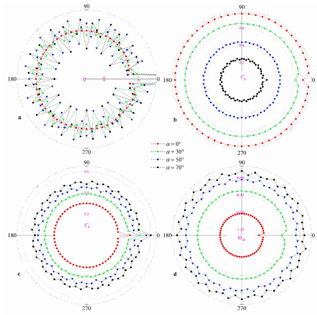
**Figure 8.** Distribution of (a) mass-flow-rate ratio  $\eta$ , (b) total-pressure-loss coefficient  $C_p$ , (c) discharge coefficient of holes  $C_d$ , and (d) adiabatic effectiveness  $\Theta_{ad}$  for different pre-swirl angles  $\alpha$ .
