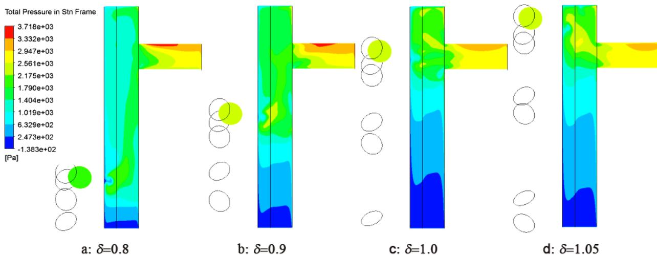
**Figure 22.** Contour of total pressure in the static frame at plane  $\theta = -12^\circ$  for different radius ratios of nozzles to holes: (a)  $\delta = 0.8$ , (b)  $\delta = 0.9$ , (c)  $\delta = 1.0$ , (d)  $\delta = 1.05$ .
