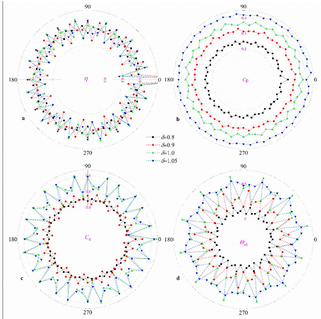
**Figure 20.** Distribution of (a) mass-flow-rate ratio  $\eta$ , (b) total-pressure-loss coefficient  $C_p$ , (c) discharge coefficient of holes  $C_d$ , and (d) adiabatic effectiveness  $\Theta_{ad}$  for different radius ratios of nozzles to holes  $\delta$ .
