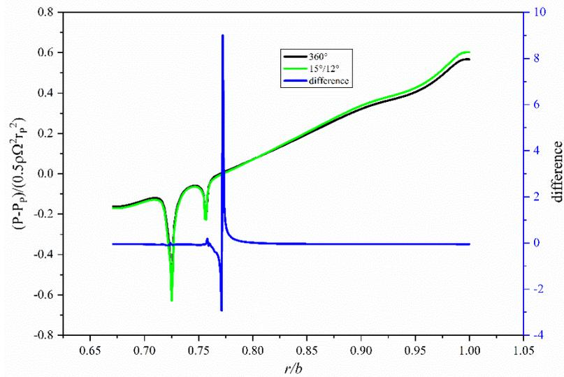
Figure 7. Profile of static pressure near stator for different models.
