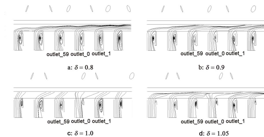
**Figure 21.** Streamlines at the cylindrical surface  $r^* = 0.926$  for different radius ratios of nozzles to holes: (a)  $\delta = 0.8$ , (b)  $\delta = 0.9$ , (c)  $\delta = 1.0$ , (d)  $\delta = 1.05$ .
