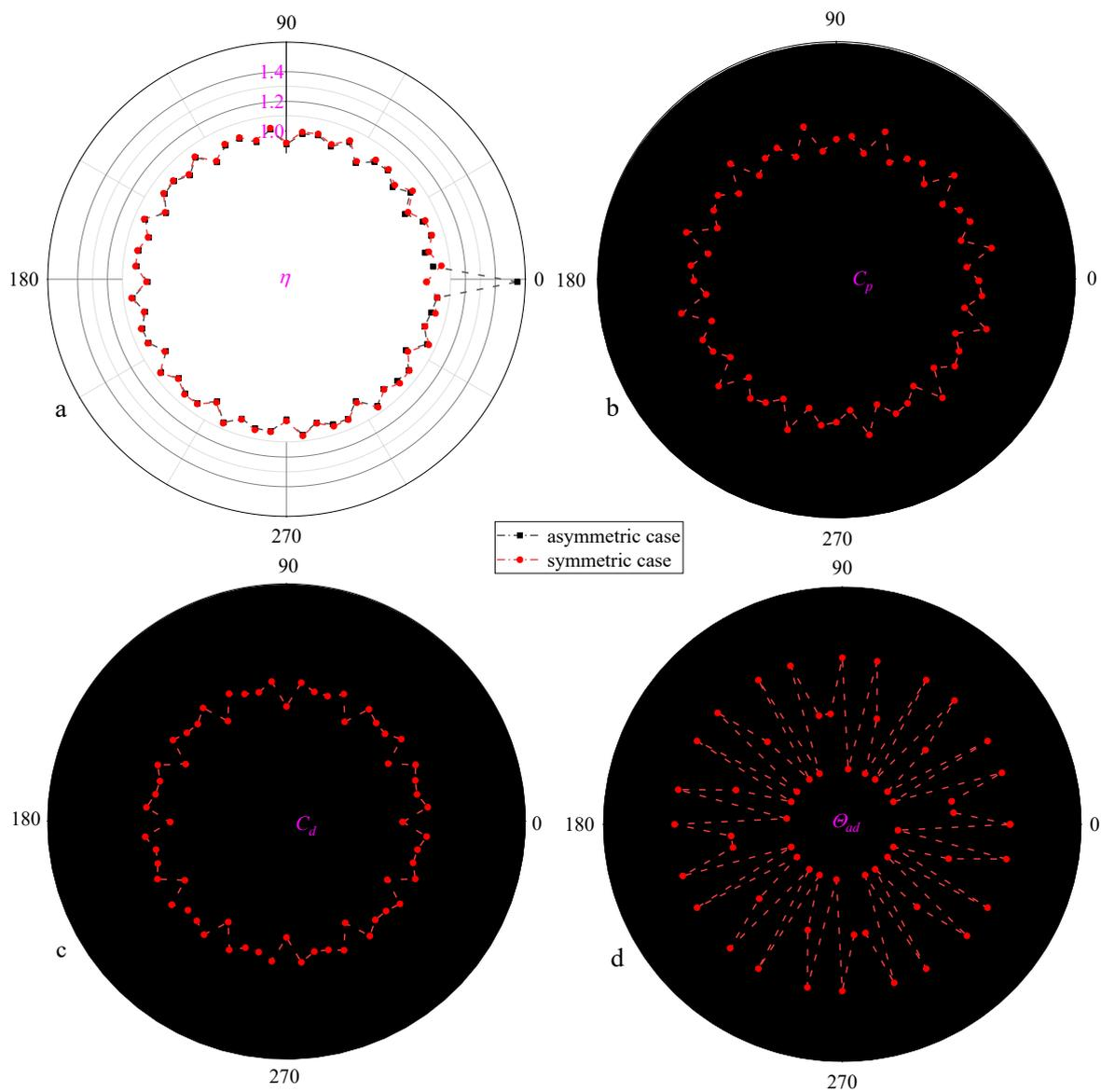
**Figure 9.** Distribution of (a) mass-flow-rate ratio  $\eta$ , (b) total-pressure-loss coefficient  $C_p$ , (c) discharge coefficient of holes  $C_d$ , and (d) adiabatic effectiveness  $\Theta_{ad}$  for symmetric and asymmetric boundary conditions when  $\alpha = 70^\circ$ .
