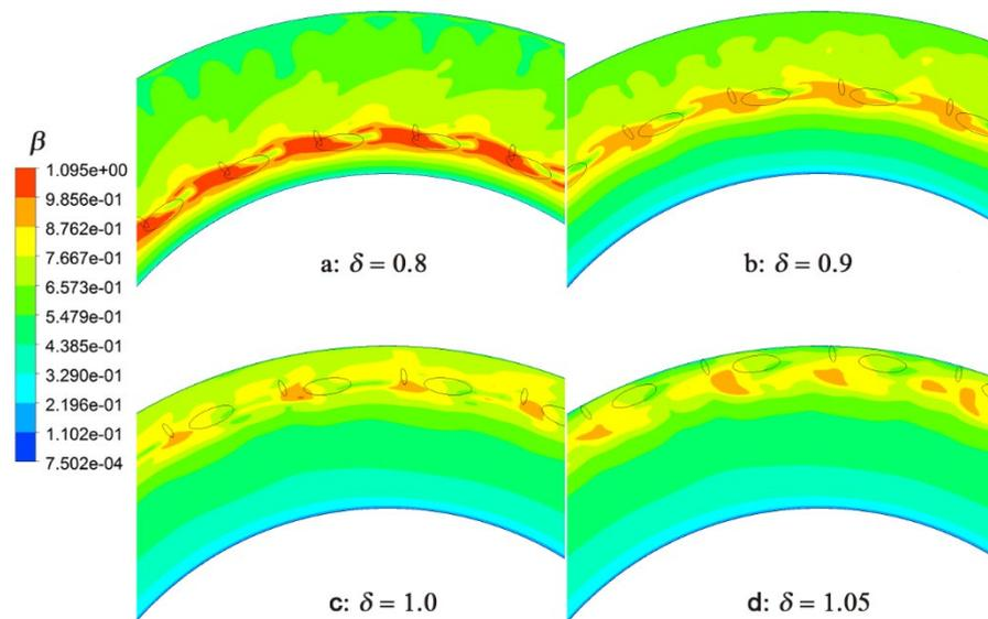
**Figure 23.** Contour of swirl ratio  $\beta$  at the plane  $z = 0.5$  for different radius ratios of nozzles to holes: (a)  $\delta = 0.8$ , (b)  $\delta = 0.9$ , (c)  $\delta = 1.0$ , (d)  $\delta = 1.05$ .
