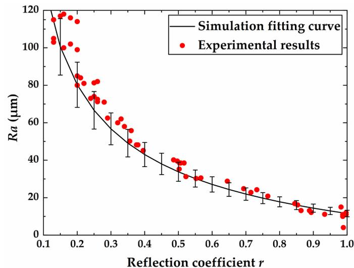
Figure 15. Experimental results for ice surface roughness in the range of [0, 120]  $\mu\text{m}$ .
