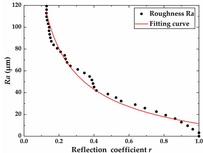
Figure 13. Corresponding relationship between roughness  $Ra$  and echo reflection coefficient  $r$ ; beads' contact angle is  $30^\circ$  and beads' height is in the range of  $[0, 370]$   $\mu\text{m}$ .
