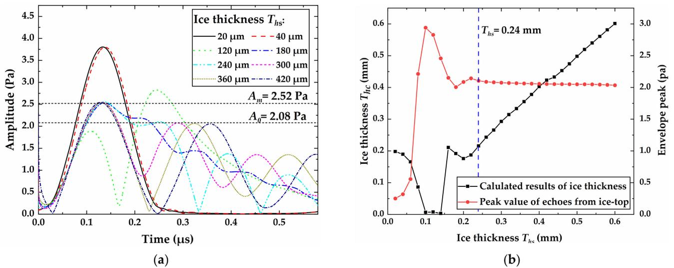
**Figure 10.** Simulation results for echo envelopes from a smooth ice top: (a) echo envelopes for different ice thicknesses; (b) ice thickness and envelope peak.
