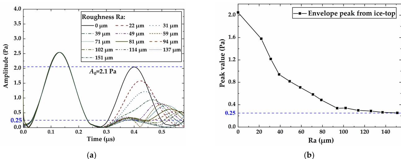
**Figure 11.** Simulation results for echo envelopes with roughness varying from 0 to 151  $\mu\text{m}$ : (a) Echo envelopes; (b) peak value.
