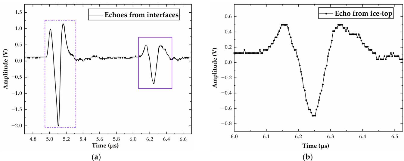
**Figure 9.** Data obtained from test with surface roughness of  $Sa = 40 \text{ }\mu\text{m}$ . The pulse in the dot-dashed rectangle is the first echo from the substrate–ice interface, and the pulse in the solid rectangle is the first echo from the top of the ice. (a) Experimental echo waveform. (b) Waveform from top of ice.
