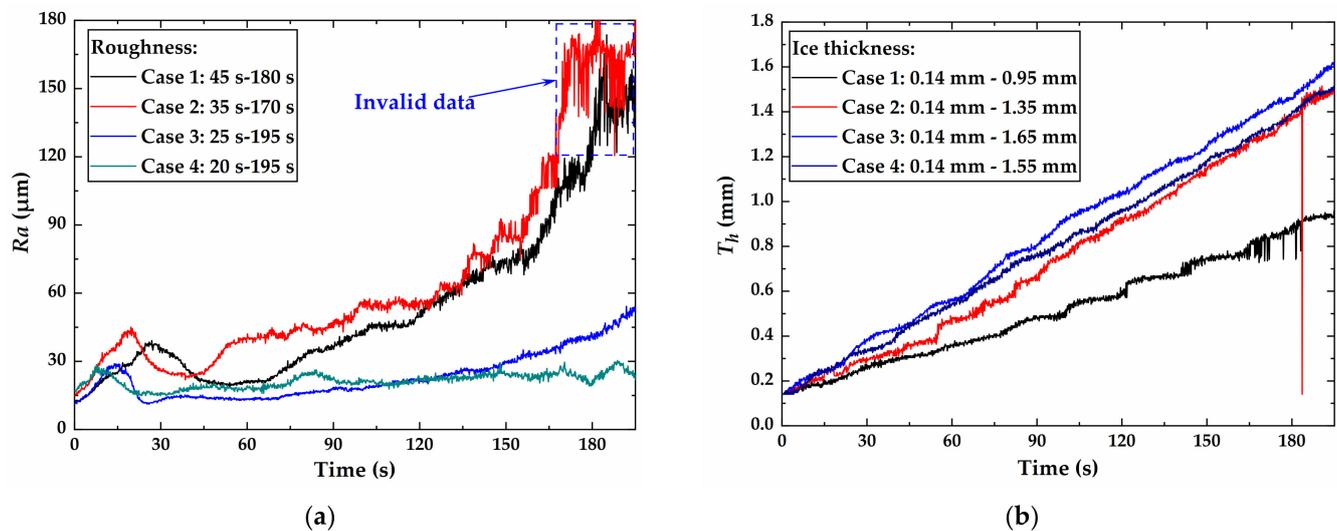
**Figure 17.** Experimental results from the icing research tunnel: (a) the growth process of the ice layer, and (b) the variation in surface roughness on the ice layer.
