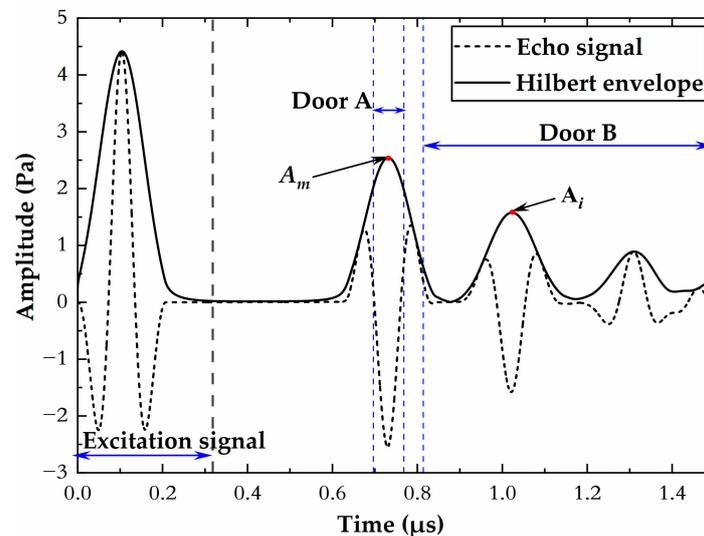
Figure 5. The original pulse-echo signal and its envelope at the interface of multilayer media.
