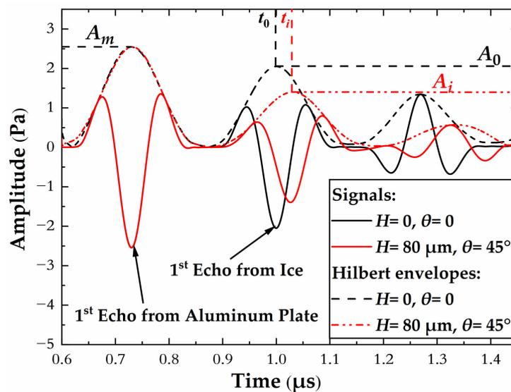
**Figure 4.** Radiofrequency echo signals (solid lines) with their envelopes (dashed lines) for an ice layer of thickness 0.5 mm. The black lines are for standard signals without roughness profiles, and the red lines are for a roughness height and a contact angle of 80 μm and 45°, respectively.
