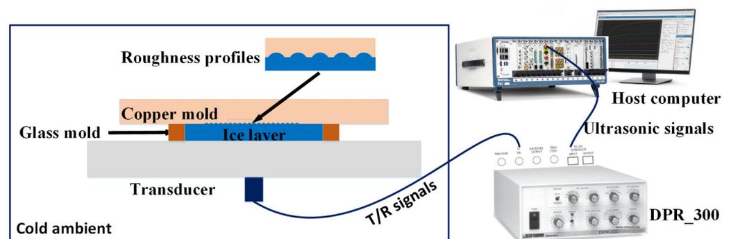
**Figure 6.** Experimental setup for measurement of roughness  $R_a$  via UPE method.
