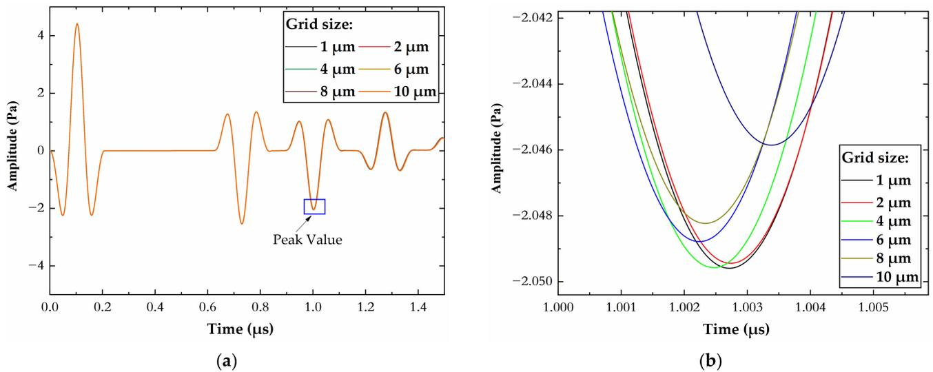
**Figure 3.** Simulation results of different grid sizes when the bead height is 10 μm: (a) Echo signals. (b) Partial enlarged view of reflected wave at the top of the ice layer.
