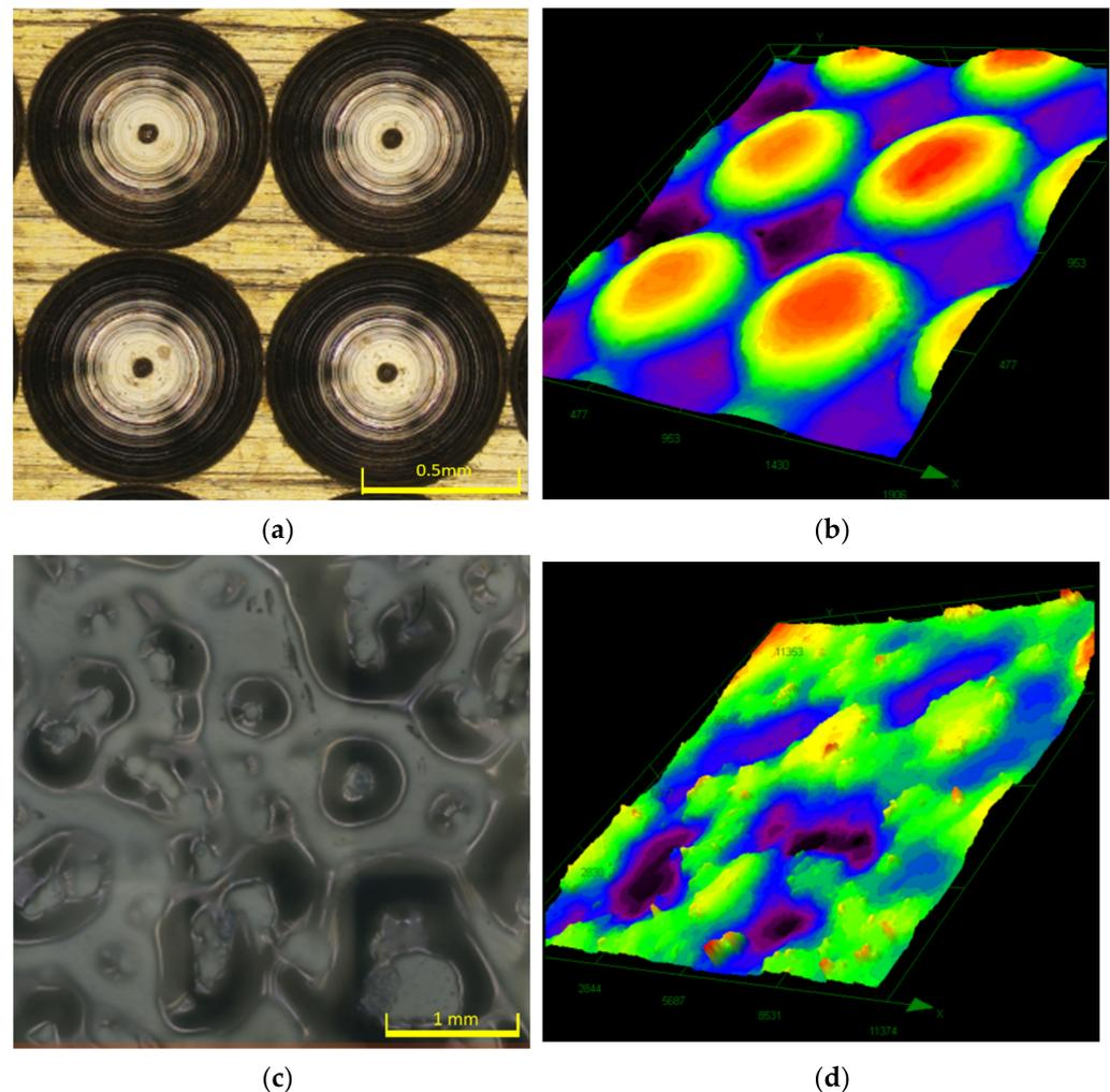
**Figure 7.** Small-scale ice roughness samples and copper molds measured by Olympus DSX-1000 microscope: (a) copper mold with spherical holes; (b) the three-dimensional contours of the regular bead ice sample; (c) glass mold with irregular roughness profile; (d) the three-dimensional contours of the irregular surface ice sample.
