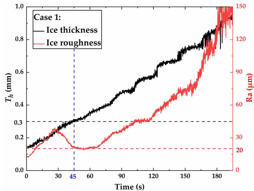
**Figure 16.** The experimental results of case 1, where the black solid line is the growth process of ice thickness, and the red solid line is the variation in ice surface roughness.
