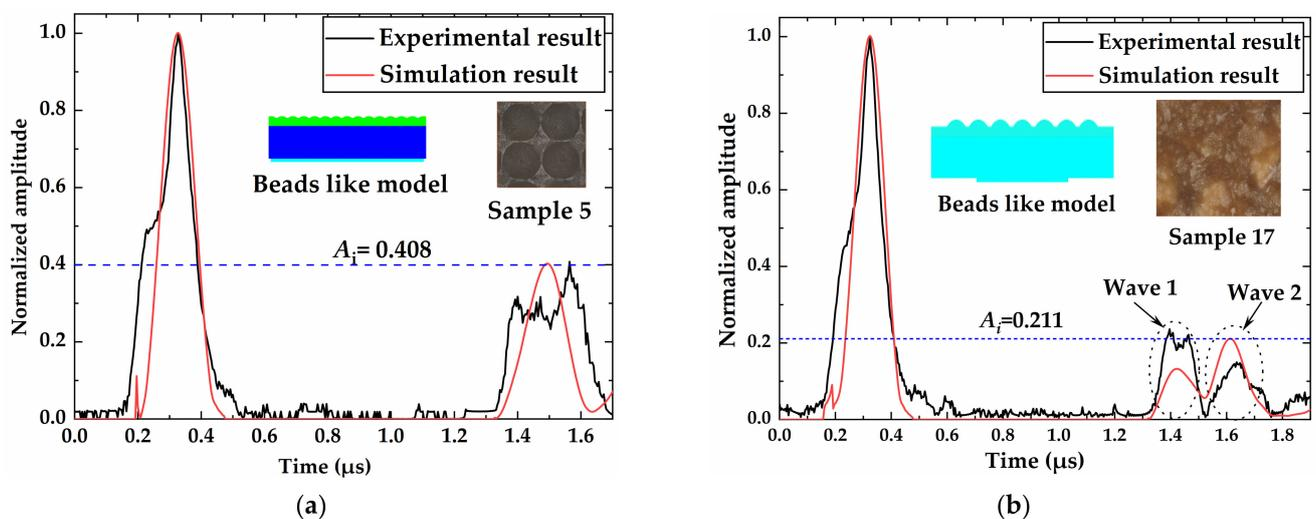
**Figure 14.** Comparison between experimental and simulated envelopes of echo signals: (a) echoes from top of ice with regular bead profile and with  $Ra = 38.5 \mu\text{m}$  and  $Sa = 39.5 \mu\text{m}$ ; (b) echoes from bead-like profile with  $Ra = 108 \mu\text{m}$  and irregular roughness profile with  $Sa = 108.8 \mu\text{m}$ .
