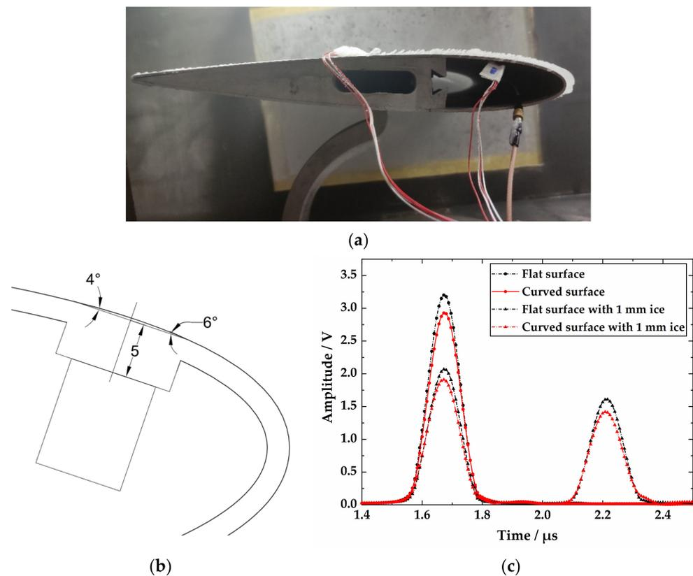
**Figure 8.** Installation of the ultrasonic transducer on NACA0012 airfoil model: (a) airfoil model in the icing wind tunnel, (b) schematic diagram of the transducer's installation position, and (c) the envelopes of echoes.
