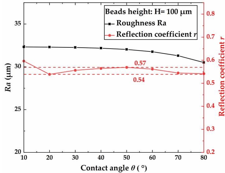
Figure 12. Numerical simulation results of roughness  $Ra$  and reflection coefficient  $r$  vs. contact angle.
