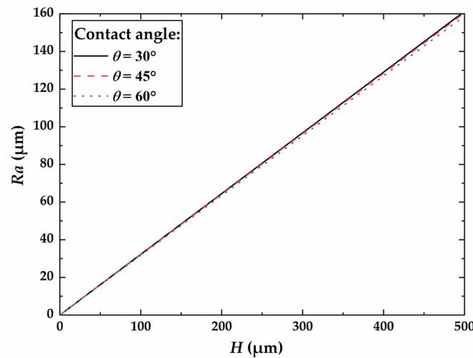
**Figure 2.** Variation in roughness with bead height at different contact angles.
