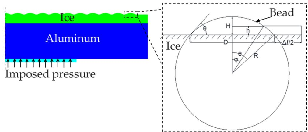
Figure 1. Schematic of a simplified 2-D symmetrical finite element model with bead-like roughness on an ice surface.
