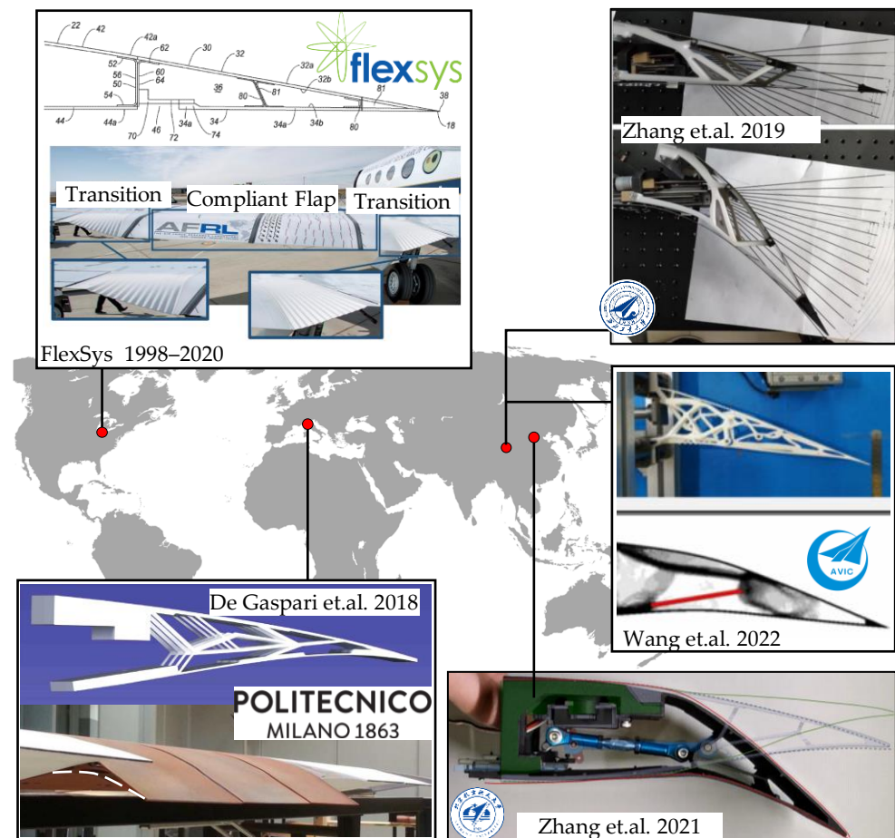
Figure 1. Trailing edge morphing solution by compliant mechanisms [1,34–39].
