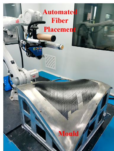
Figure 13. Automated fiber placement experimental platform.
