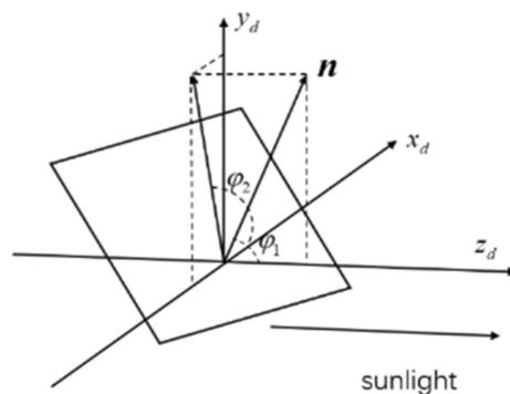
**Figure 3.** Solar sail body coordinate system.
