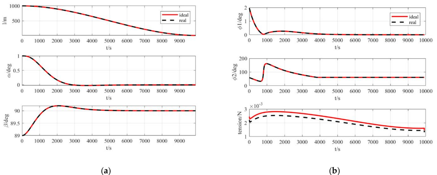
**Figure 7.** (a) State trajectory during the retrieval of a satellite-sail system; (b) control input trajectory during the retrieval of a satellite-sail system.
