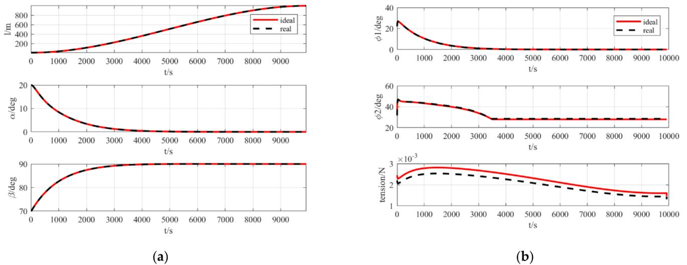
**Figure 6.** (a) State trajectory during the deployment of a satellite-sail system; (b) control input trajectory during the deployment of a satellite-sail system.
