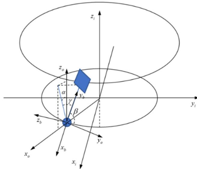
**Figure 2.** Definition of coordinate systems for traverse formation.
