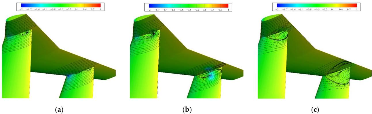
**Figure 12.** Streamlines and  $C_p$  distribution on the suction side of the vertical tail parts:  $\beta =$  (a)  $0^\circ$ , (b)  $2^\circ$ , and (c)  $4^\circ$ .
