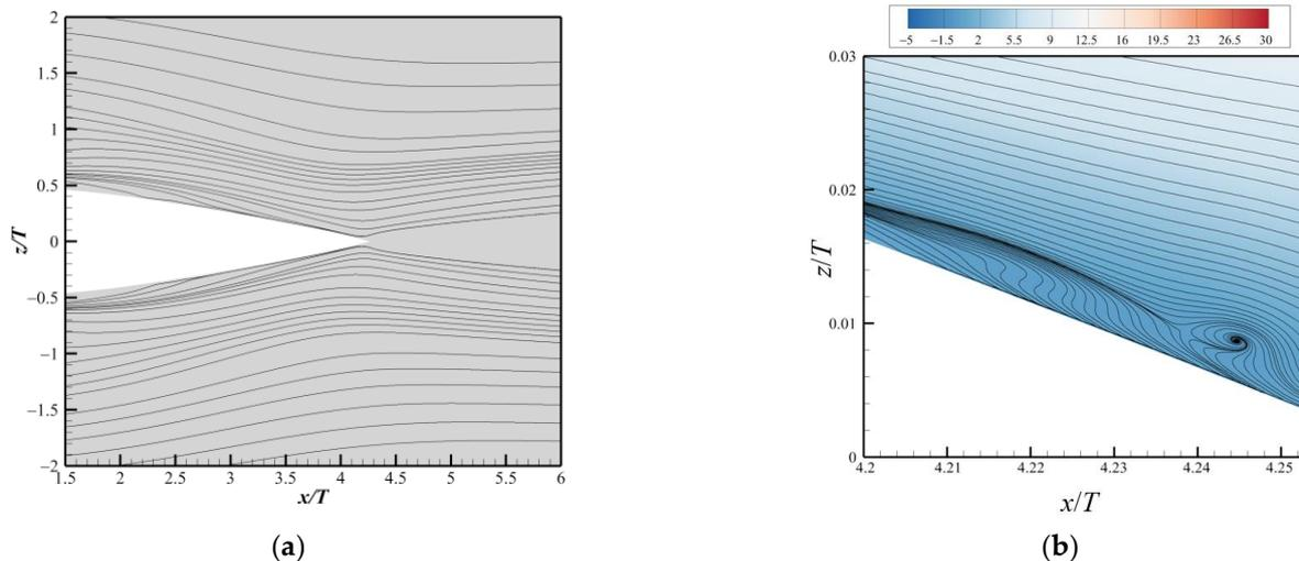
**Figure 7.** Streamlines on bottom wall calculated using SLA-IDDES: (a) streamlines with a fishtail shape at trailing edge; (b) flow separation at the trailing edge, colored by the streamwise velocity.
