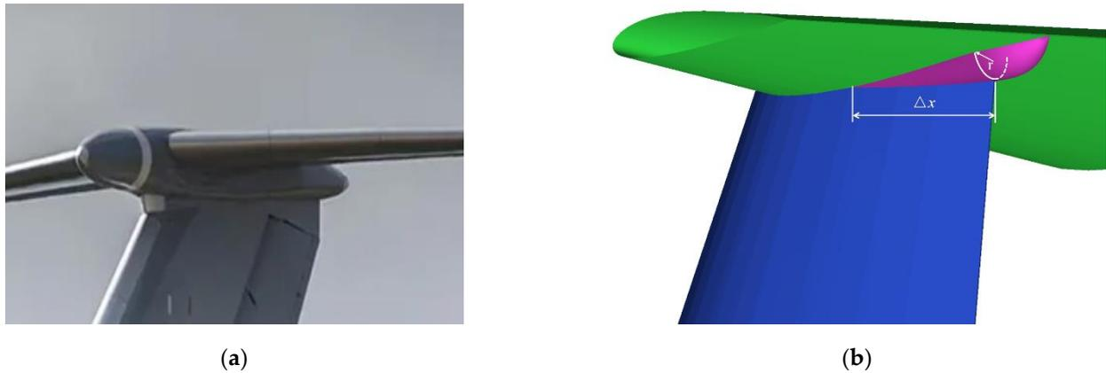
**Figure 15.** Two different fairing-cone models: (a) bullet fairing cone; (b) schematic of the fairing cone model used herein.
