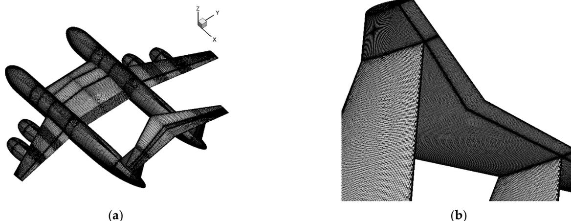
**Figure 9.** (a) Surface mesh of whole demonstration aircraft with a coarse grid. (b) Surface mesh of the T-tail with a fine grid.
