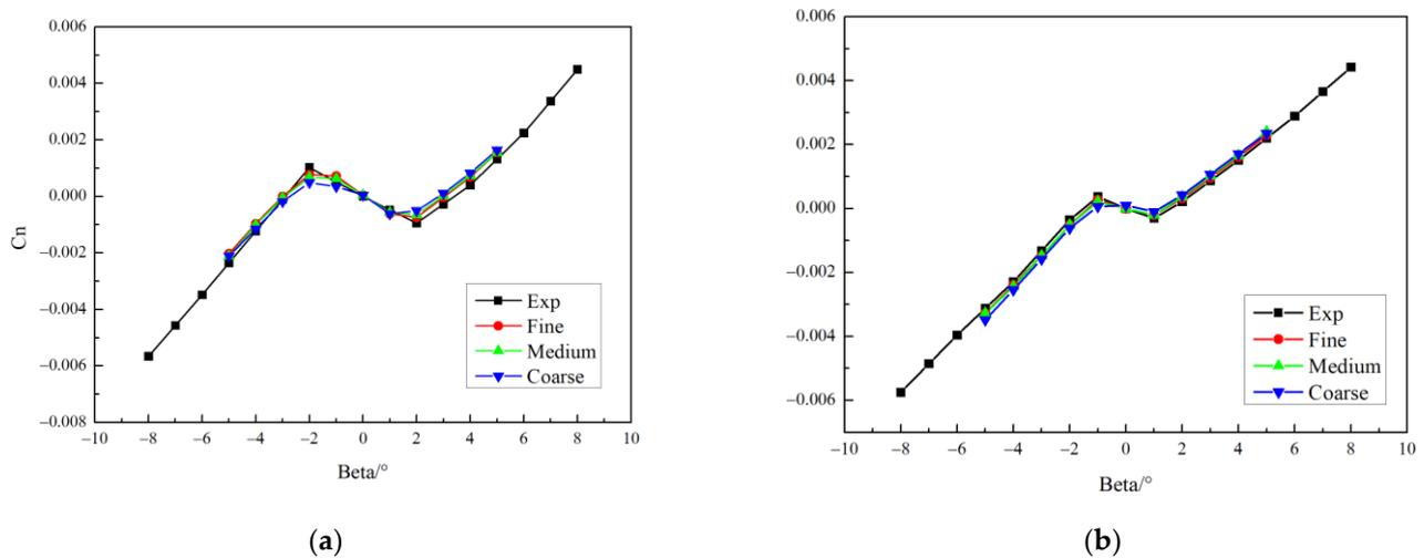
**Figure 10.** Coefficient of yaw moment calculated with three different grids, and comparison with the experimental results. (a)  $\alpha = 0^\circ$  (b)  $\alpha = -4^\circ$ .
