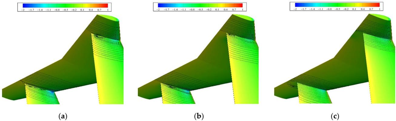
**Figure 11.** Streamlines and  $C_p$  distribution on the pressure side of the vertical tail parts:  $\beta =$  (a)  $0^\circ$ , (b)  $2^\circ$ , and (c)  $4^\circ$ .
