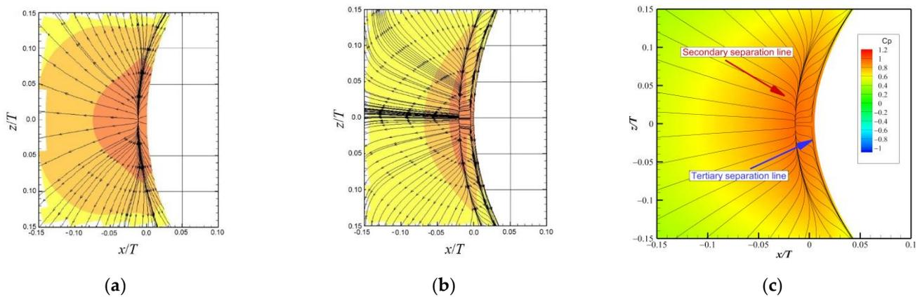
**Figure 6.** Secondary and tertiary separation lines on the bottom wall: (a) RANS/LES [27]; (b) wall-resolved LES [31]; (c) SLA-IDDES.
