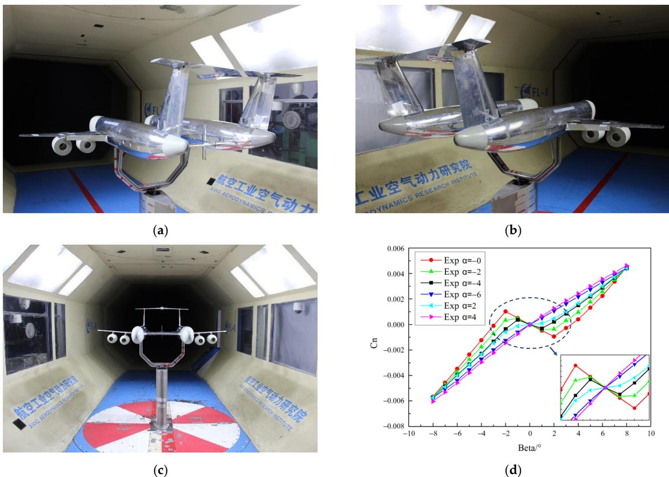
**Figure 8.** Experimental model of the demonstration aircraft in a wind tunnel: (a) left side of the aircraft; (b) right side of the aircraft; (c) front of the aircraft; (d) results for coefficient of yaw moment.
