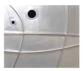
Figure 16. The fully-dense additive components with AFSD [62].
