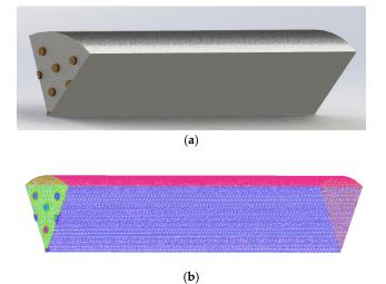
Figure 2. The 1/6 combustor structure. (a) Computational domain. (b) Computational grid.
