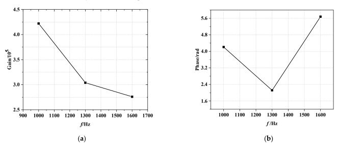
**Figure 8.** Central injector flame transfer function. (a) Amplitude–frequency curve. (b) Phase–frequency curve.
