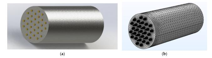
Figure 9. (a) Geometry of a compact flame. (b) Unstructured mesh of the acoustic field solution.
