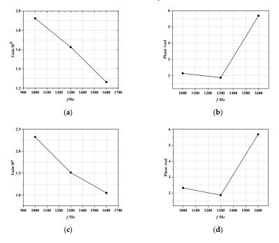
**Figure 11.** The flame transfer function of the central injector. (**a**) The amplitude–frequency curve of Scheme 7. (**b**) The phase-frequency curve of the Scheme 7. (**c**) The amplitude–frequency curve of Scheme 8. (**d**) The phase–frequency curve of the Scheme 8.
