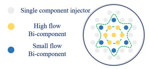
Figure 3. Injector distribution in the injection panel.
