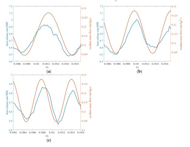
**Figure 10.** The relationship between the sum of heat release rate and inlet flow rate pulsation. (a) 1000 Hz. (b) 1300 Hz. (c) 1600 Hz.
