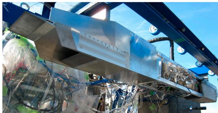
**Figure 2.** Pre-cooled turbojet engine.
