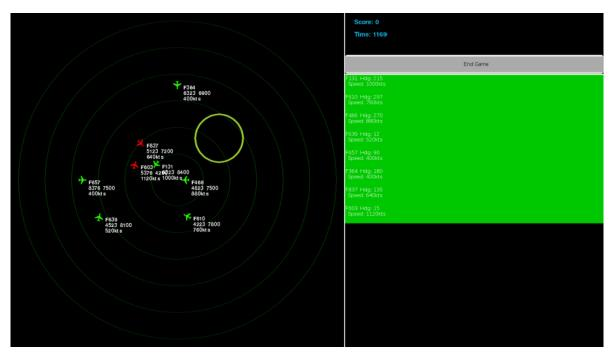
**Figure 3.** Human–computer interaction interface. A group of aircraft are generated and displayed on the left area, with specific information of each aircraft listed on the lower right area. The upper right area serves for displaying time and scores.
