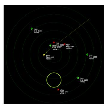
**Figure 2.** Airspace display area. Aircraft are generated randomly in green. When an aircraft is clicked, it turns yellow and the projected trajectory shows up. The aircraft turns red if it is involved in a conflict. The area covered by the green circle is the danger zone, where aircraft are not allowed to enter.
