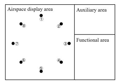
**Figure 1.** The layout of the simulation software's interface. Aircraft are generated and displayed on the left area, with specific information of each aircraft listed on the lower right area. The upper right area serves for displaying the time and score.
