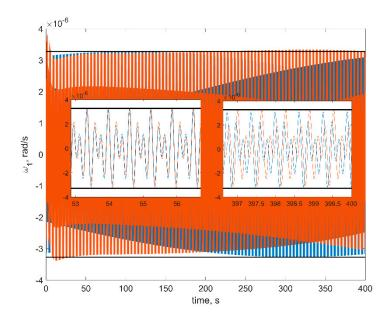
**Figure 6.** Evolution of  $\omega_1$  (red is numerical solution, blue is approximate solution, horizontal lines are the estimations).
