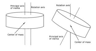
Figure 1. RW imbalances: Static (left) and dynamic (right).
