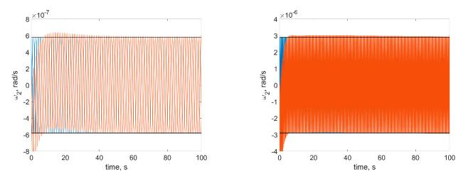
**Figure 10.** Stabilization accuracy for  $\Omega_1 = 10$  s  $^{-1}$  (left) and  $\Omega_1 = 50$  s  $^{-1}$  (right).
