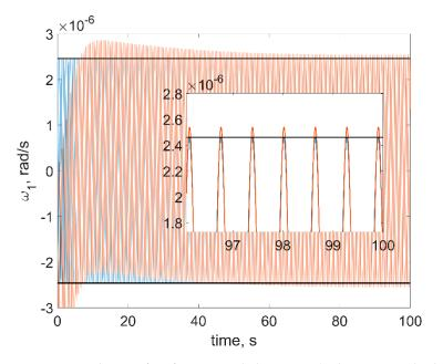
**Figure 11.** Evolution of  $\omega_1$  for static imbalance case (red is numerical solution, blue is approximate solution, horizontal lines are the estimations).
