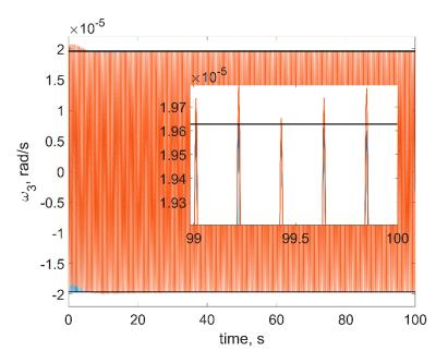
**Figure 13.** Evolution of  $\omega_3$  for static imbalance case (red is numerical solution, blue is approximate solution, horizontal lines are the estimations).
