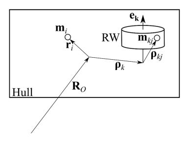
Figure 2. Spacecraft and reaction wheel.
