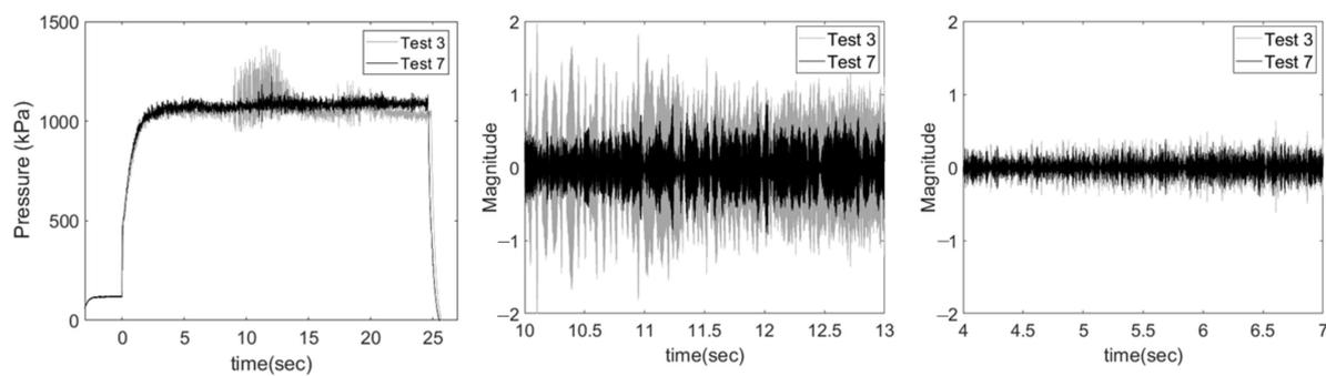
**Figure 12.** Overlays of combustion pressure and filtered pressure in tests 3 and 7.
