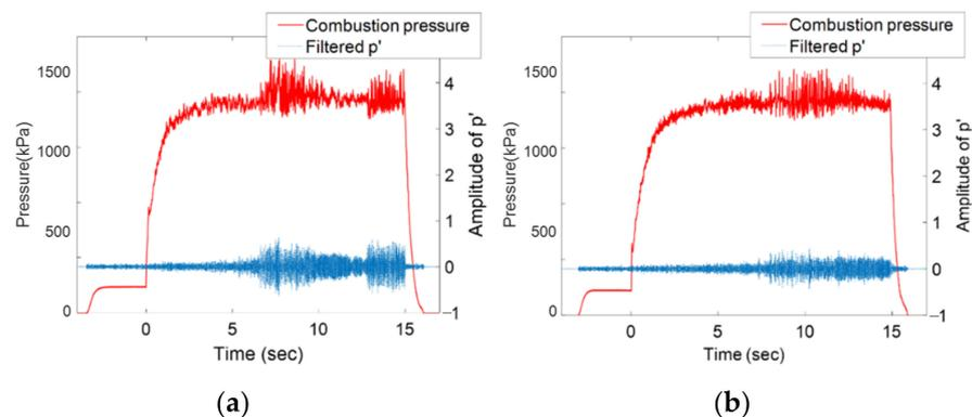
**Figure 4.** Combustion pressure and filtered pressure fluctuations  $p'$  in (a) baseline and (b) test 1.
