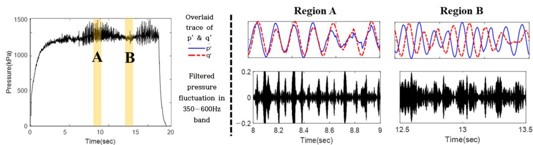
**Figure 2.** Overlays of  $p'$  and  $q'$  (top row) in regions A and B (left) and filtered from 350 to 600 Hz (bottom row).
