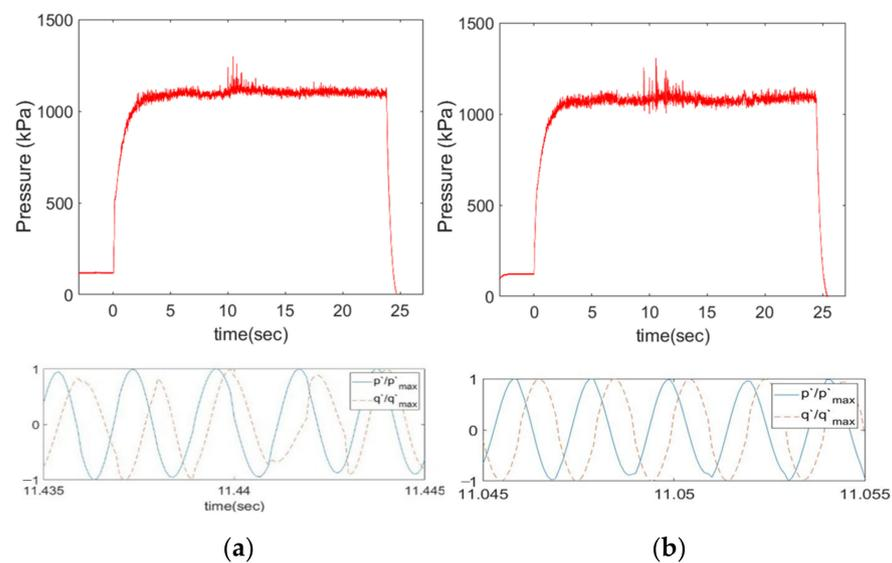
**Figure 11.** Combustion pressure and coupling status between normalized  $p'$  and  $q'$  in (a) test 4 ( $5^\circ$ ) and (b) test 6 ( $6^\circ$ ).
