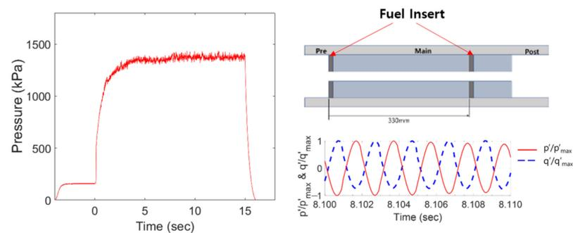
**Figure 7.** Combustion pressure and normalized  $p'$  and  $q'$  from test 2.
