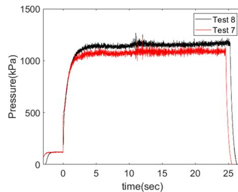
**Figure 14.** Comparison of combustion pressures in tests 7 and 8.
