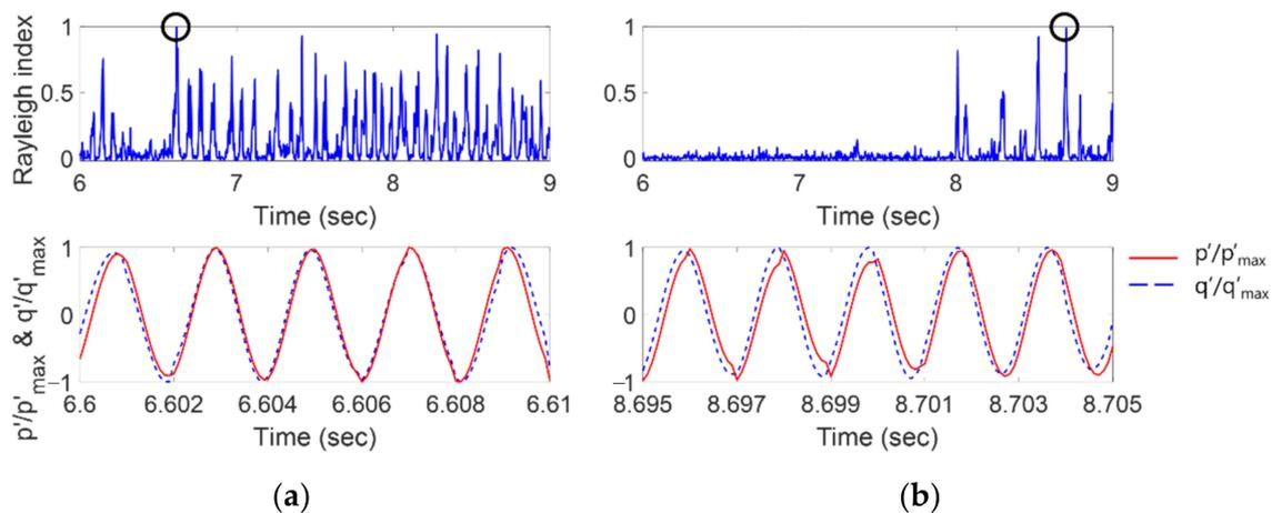
**Figure 6.** Rayleigh index (RI) and overlay of normalized  $p'$  and  $q'$  in (a) baseline and (b) test 1.
