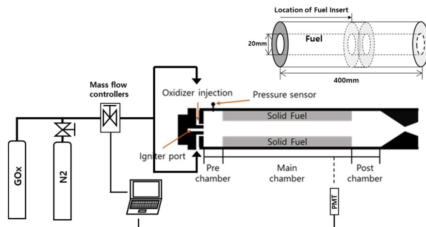
**Figure 3.** Schematic of test configuration and PMT setup for image capturing.
