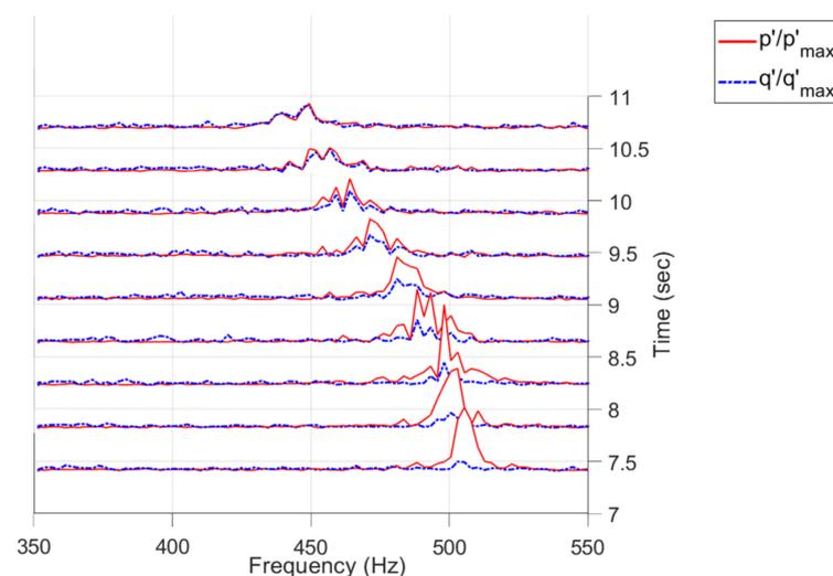
**Figure 8.** Temporal shift in frequency peaks for normalized  $p'$  and  $q'$  from test 2.
