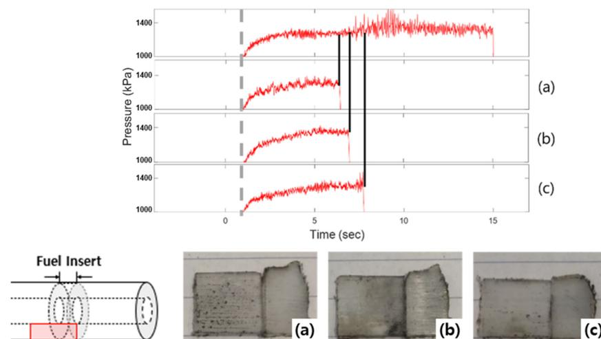
**Figure 5.** Sequential images of fuel cross section and corresponding pressure traces in test 1 up to (a) 6.4 s, (b) 7.6 s, and (c) 8.4 s.
