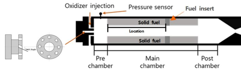
**Figure 9.** Schematic of combustion test setup.
