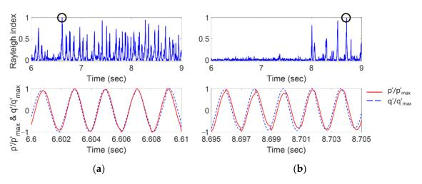
**Figure 6.** Rayleigh index (RI) and overlay of normalized p' and q' in (**a**) baseline and (**b**) test 1.
