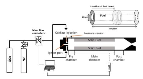
Figure 3. Schematic of test configuration and PMT setup for image capturing.
