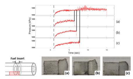
**Figure 5.** Sequential images of fuel cross section and corresponding pressure traces in test 1 up to (a) 6.4 s, (b) 7.6 s, and (c) 8.4 s.
