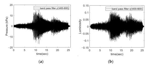
**Figure 10.** Filtered traces of (**a**) pressure (p') and (**b**) luminosity fluctuations (q') in test 3.
