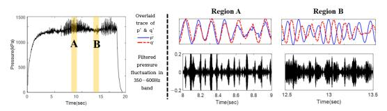
**Figure 2.** Overlays of p' and q' (top row) in regions A and B (left) and filtered from 350 to 600 Hz (bottom row).
