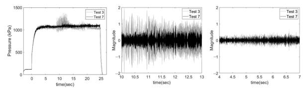
Figure 12. Overlays of combustion pressure and filtered pressure in tests 3 and 7.
