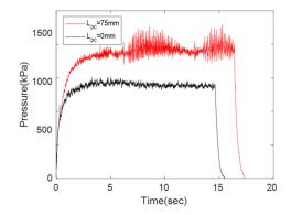
Figure 1. Comparison of combustion pressures with and without the post chamber.
