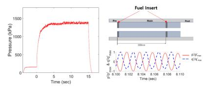
**Figure 7.** Combustion pressure and normalized p' and q' from test 2.
