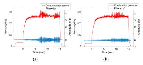
**Figure 4.** Combustion pressure and filtered pressure fluctuations p' in (**a**) baseline and (**b**) test 1.
