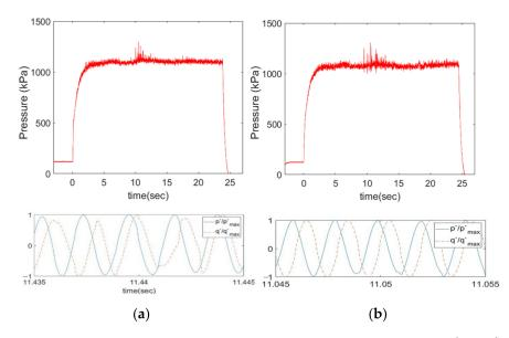
**Figure 11.** Combustion pressure and coupling status between normalized p' and q' in (**a**) test 4 (5°) and (**b**) test 6 (6°).
