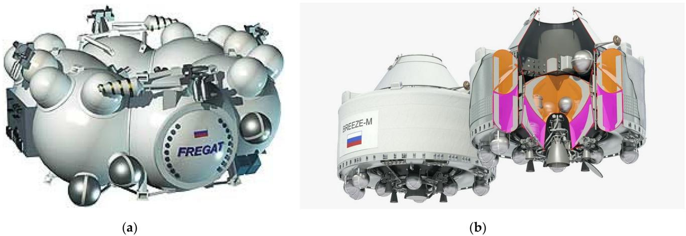
**Figure 2.** Examples of liquid propelled space tugs: (a) NPO Lavochkin Fregat (Soyuz/Zenit); (b) GKNPTs Khrunichev Briz-M (Proton). Note the extremely compact length to diameter ratio and the propellant tank arrangement. Copyright: publicly available pictures on the internet.
