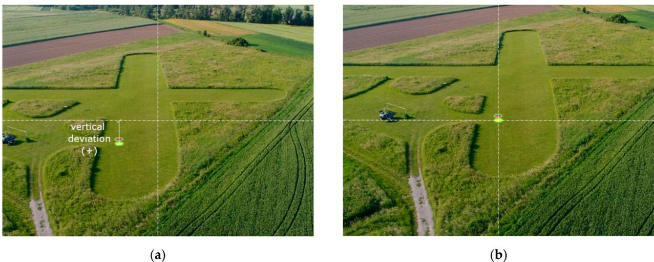
**Figure 4.** Samples of pictures gathered by the on-board camera with marked dedicated runway signs system; (a) incorrect configuration; (b) correct configuration-aircraft is aiming the signs system. Crossed dash-dot lines mark the center of the image and the real aiming point.
