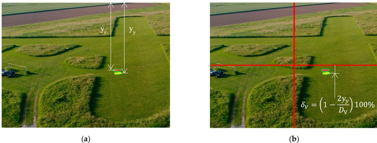
**Figure 7.** (a) Identified and contoured ground signs system appearing to the on-board vision system with marked centers of circles; (b) yellow circle's relative position  $\delta_V$  to the horizontal center of the picture,  $D_V$  is the height of the picture in pixels.
