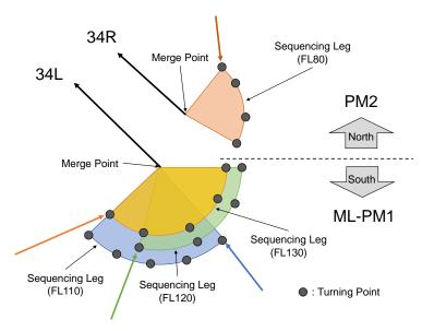
**Figure 6.** Schematic diagram of the configuration of the point-merge (PM) system connected to 34L (multi-level point merge 1: ML-PM1) and 34R (point merge 2: PM2) in Tokyo Approach Control Area (TACA) with northerly wind operation.
