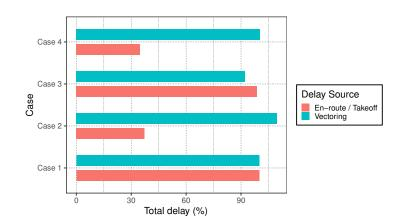
**Figure 17.** Comparing the increase in the total delay in arrival air traffic as a whole at runway 34L in RJTT.
