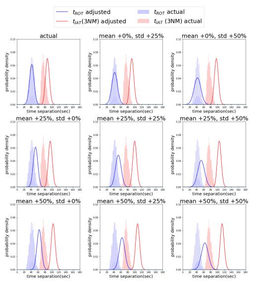
**Figure 9.** Nine cases of  $t_{ROT}$  distributions (**blue**) and  $t_{IAT}$  distributions of arrival aircraft pairs with a separation minimum of 3 NM (**red**) that maximize the runway capacity while satisfying the ROT constraints in each case.
