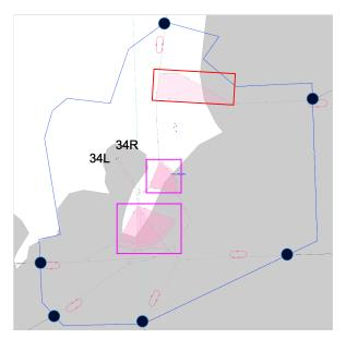
**Figure 13.** TACA (blue polygon) and two runways (34L and 34R) at RJTT. Vectoring zones are composed of an red rectangle (radar vector) and pink rectangle (point-merge system). The traffic volumes in TACA and in-trail separation at entry fixes are assumed in the simulation.
