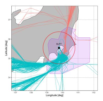
**Figure 5.** Actual radar tracks bound for RJTT coming from a northern direction (orange lines) and southern direction (blue lines) in the northerly wind operation in a day in October 2019. Tokyo Approach Control Area (TACA) is bounded by a purple polygon. The radius of the red circle is 50 NM centered on RJTT.
