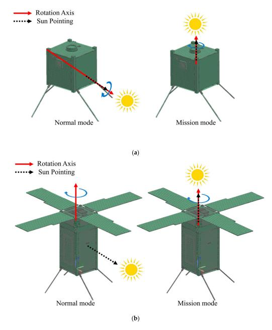
Figure 9. Attitude of CubeSats on the normal and mission mode: (a) Timon; (b) Pumbaa.
