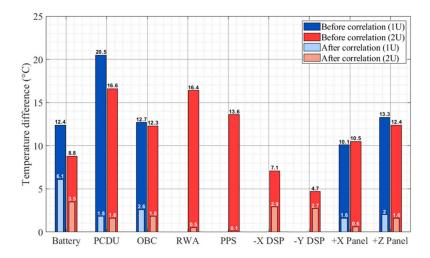
**Figure 23.** Temperature difference between the TVCT and the numerical analysis before and after the correlation.
