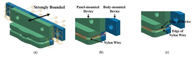
**Figure 19.** Three types of nylon wire tightening in the HRM of the Pumbaa: (**a**) Strongly bounded; (**b**) Nylon wire connected to edge of device; (**c**) Edge of nylon wire connected to edge of device.
