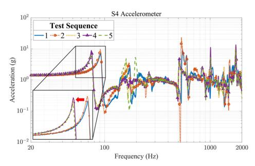
Figure 18. Change in natural frequency along the X-axis LLSS test as test sequence.
