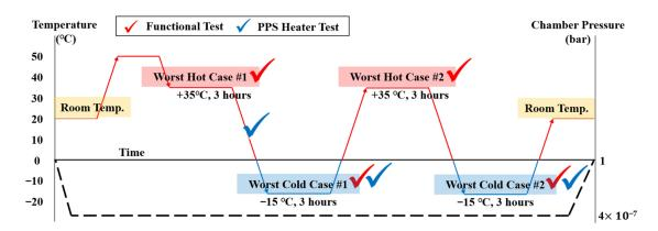
Figure 16. Temperature profile and procedure of TVCT.
