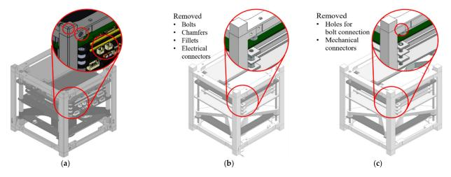
**Figure 3.** CAD and analytical models: (a) Detailed CAD model and (b) structural and (c) thermal analytical models of Timon.
