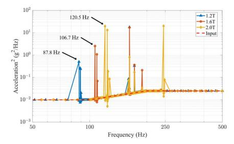
**Figure 6.** Natural frequencies ( $f_0$ ) along the +Y-axis of the DSP in the axial direction with different DSP thicknesses.
