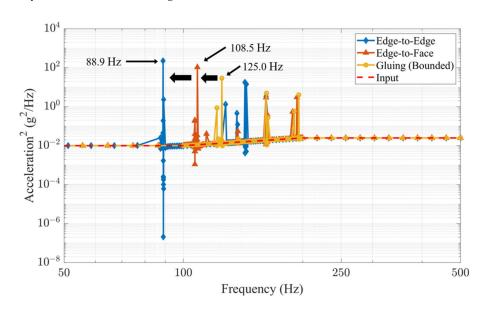
Figure 20. 1st mode natural frequency shifts as constraint level changes.
