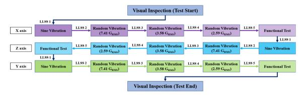
Figure 14. Vibration testing flow diagram.
