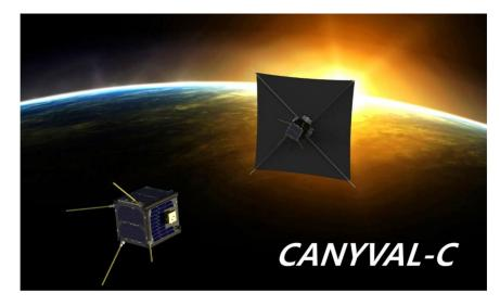
**Figure 1.** Concept of CANYAL-C mission [4]. The CubeSat on the left is Timon (1U CubeSat) and that on the right, with a deployed occulter, is Pumbaa (2U CubeSat).
