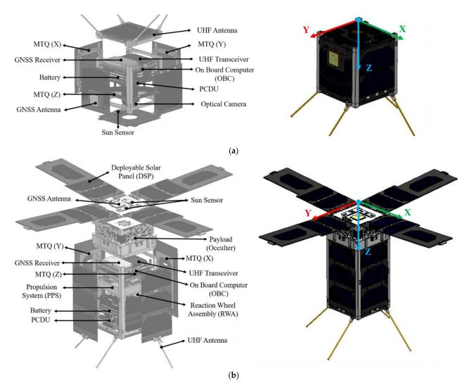
Figure 2. CubeSat hardware configuration and coordinate system: (a) 1U CubeSat, Timon; (b) 2U CubeSat, Pumbaa.
