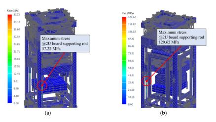
**Figure 8.** Random vibration and shock analysis results: (**a**) random vibration (maximum stress in Y-axis); (**b**) shock (maximum stress in X-axis).
