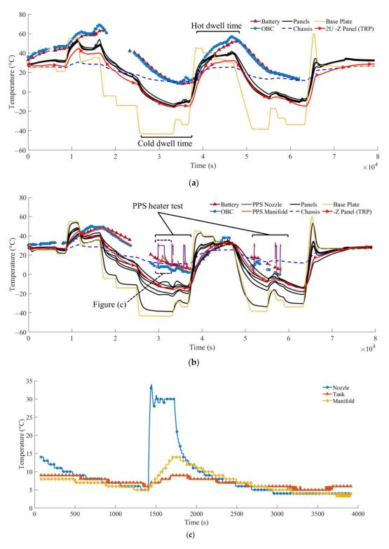
**Figure 21.** TVCT results: (a) Timon temperature profile; (b) Pumbaa temperature profile; (c) PPS temperature profile of Pumbaa during heater activation.
