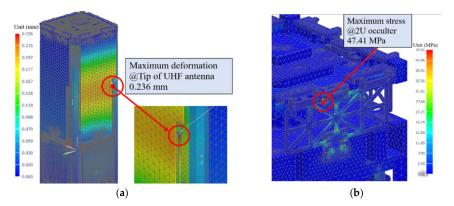
**Figure 7.** Quasi-static acceleration analysis results: (**a**) maximum deformation in X-axis; (**b**) maximum stress in Y-axis.
