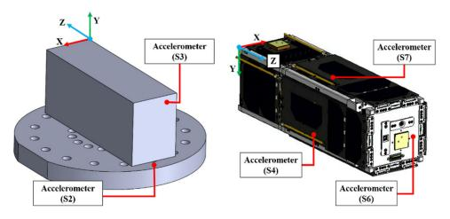
**Figure 12.** Accelerometer attachment locations. The three accelerometers were located in Pumbaa's –X-axis DSP, –Y-axis DSP, and +Z-axis panel. The other two accelerometers were located in the test P-POD and fixture.
