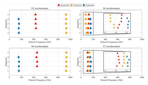
**Figure 17.** Modal survey results of the natural frequencies. The S3, S4, S6, and S7 accelerometers are located in the T-POD, –X-axis DSP of Pumbaa, –Y-axis DSP of Pumbaa, and +Z-axis panel of Pumbaa, respectively.
