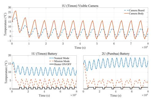
Figure 11. Temperature of visible camera and battery and operation of battery heater.
