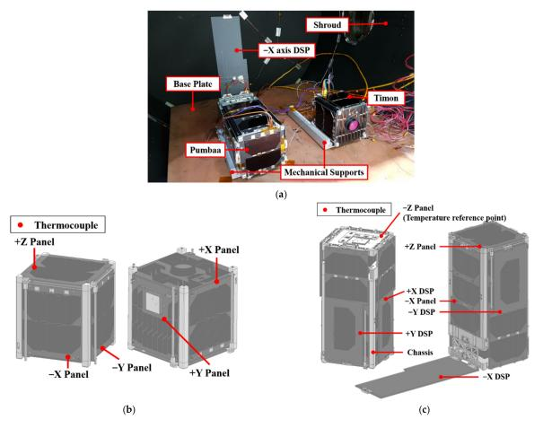
Figure 15. TVCT setting: (a) CubeSat arrangement in the chamber; (b) TCs on Timon; (c) TCs on Pumbaa.
