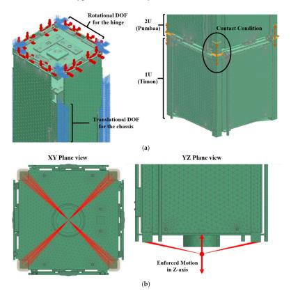
**Figure 5.** Analysis condition settings: (**a**) DOF constraints and contact conditions; (**b**) XY Plane view and YZ plane view of enforced motion for Z-axis modal analysis.
