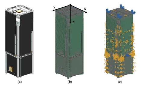
**Figure 4.** Models for the analyses: (a) Simplified CAD models of two CubeSats contained in the deployer; (b) 3-D tetrahedral type model; (c) Analytical model with contact conditions and DOF conditions.
