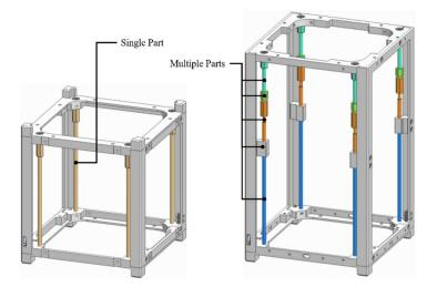
Figure 24. Configuration of board supporting rods of CubeSats (left: Timon, right: Pumbaa).
