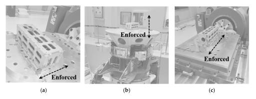
Figure 13. Vibration testing configuration: (a) X-axis test; (b) Y-axis test; (c) Z-axis test.
