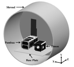
**Figure 22.** Duplicated thermal vacuum chamber and the CubeSats for the correlation of the TVCT parameters.
