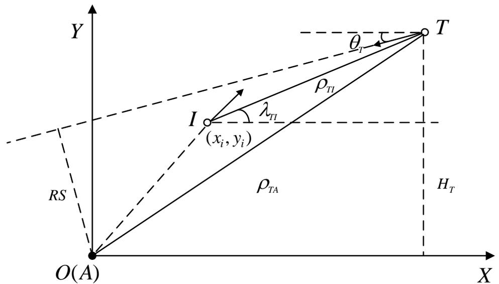
Figure 2. The planar geometry of the interceptor, target and defending asset.
