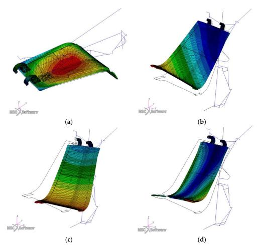
**Figure 10.** Normal modes of an MLG door baseline configuration: closed door (**a**) main flexural mode f = 200 Hz; open door (**b**) harmonic mode, f = 20.6 Hz; (**c**) fore and aft mode, f = 36 Hz; and (**d**) torsional mode, f = 52.4 Hz.
