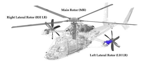
Figure 1. Racer rotorcraft view: details of the vibration sources [33].
