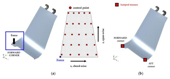
**Figure 11.** MLG door analysis setup: (a) dynamic load application and virtual acquisition points on MLG door; (b) ballast mass position.
