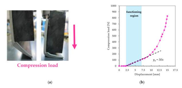
**Figure 9.** Stiffness characterization of leap seal: (a) compression test; (b) linear ( $K_{seal} = 50 \text{ N/mm}$ ) and nonlinear load-ing curves.
