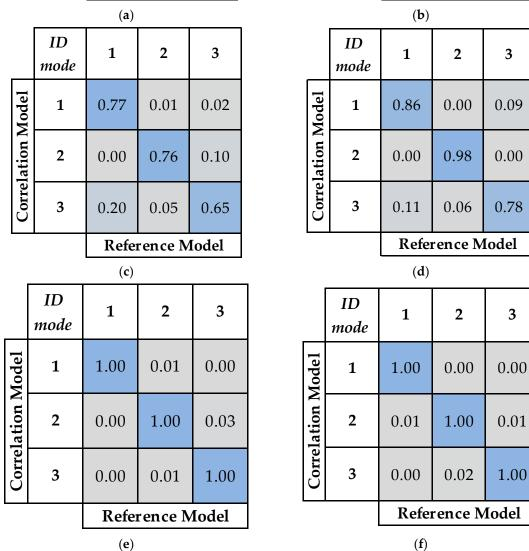
**Figure 16.** Mode shape orthogonalization verification with respect to the baseline configuration: (**a**) 0.5 kg on each side; (**b**) 1 kg on the forward corner; (**c**) 1 kg on the aft corner; (**d**) pushrod link failure; (**e**) pulling down aero pressure; and (**f**) pushing up aero pressure.
