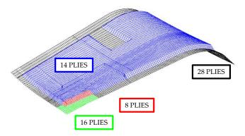
Figure 6. Laminate FE model: mapping of plies distribution.
