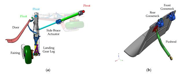
**Figure 2.** Main landing gear (MLG) system architecture: (**a**) door and fairing with the actuation system; (**b**) MLG door with a focus on the metallic gooseneck connecting the door to the airframe and the pushrod linking the door to the LG (Landing Gear) leg.
