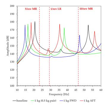
Figure 12. Extra-mass addition on an MLG door.
