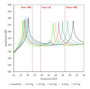
Figure 13. Tuning mass sensitivity on an MLG door.
