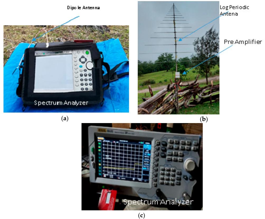
**Figure 2.** Photos of measurement: (a) Anritsu MS2721B; (b) log periodic antenna and pre amplifier; (c) Rigol DSA 815.
