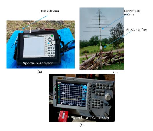
**Figure 2.** Photos of measurement: (**a**) Anritsu MS2721B; (**b**) log periodic antenna and pre amplifier; (**c**) Rigol DSA 815.
