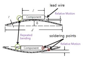
Figure 10. Relative bending motion between components and PCB.
