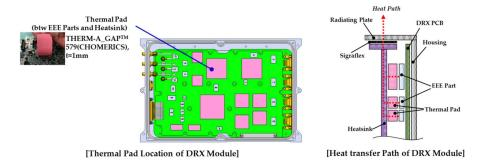
Figure 4. Schematic diagram of the thermal control strategy of DRX and HSDRU.
