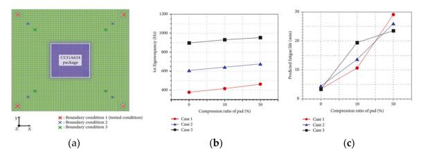
**Figure 18.** Numerical fatigue life prediction on solder joint [10]. (a) Boundary conditions for structural analysis. (b) 1st Eigen-frequency of the PCB for the compression ratio of the thermal gap pad in each case. (c) Fatigue life on solder joint for CCGA624 package with respect to the fatigue life in each case.
