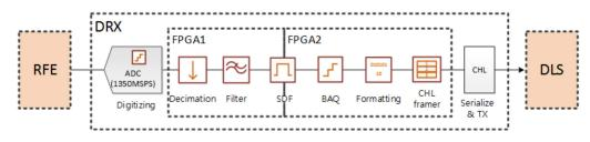
Figure 1. Functional diagram of data processing for DRX.
