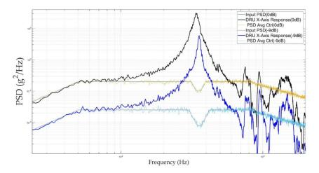
Figure 15. Random vibration test results 0 dB and -9 dB of HSDRU.
