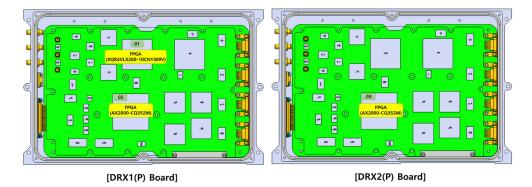
Figure 12. Component with minimum MoS in DRX.
