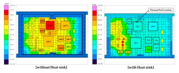
Figure 7. Temperature contours of DRX1(P) with and without heat sink.
