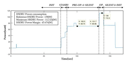
Figure 19. *x*-axis power consumption test results after *x*-axis random vibration test.
