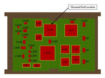
Figure 6. DRX internal configuration with heat dissipation and thermal pad location.
