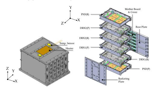
Figure 3. Mechanical configuration and exploded view of HSDRU.
