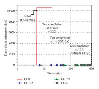
Figure 17. Time profiles of daisy-chain resistance for each specimen [10].
