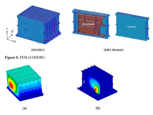
**Figure 9.** Modal analysis results of HSDRU. (**a**) First 338.9Hz (global bending mode). (**b**) Sixteenth 775.7 Hz (local mode, DRX heat sink).
