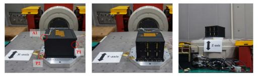
Figure 13. Vibration test configuration and accelerometer position of HSDRU.
