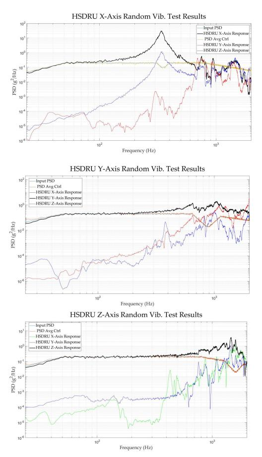
Figure 14. Random vibration test results of HSDRU about X-, Y-, and Z-axes.
