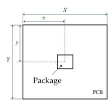
Figure 11. Location factor of component related to relative position factor of package.
