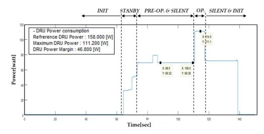
Figure 21. *x*-axis power consumption test results after *x*-axis shock test.
