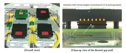
Figure 16. Random vibration fatigue test setup [10].
