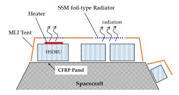
Figure 2. Schematic of thermal control strategy of HSDRU on spacecraft.
